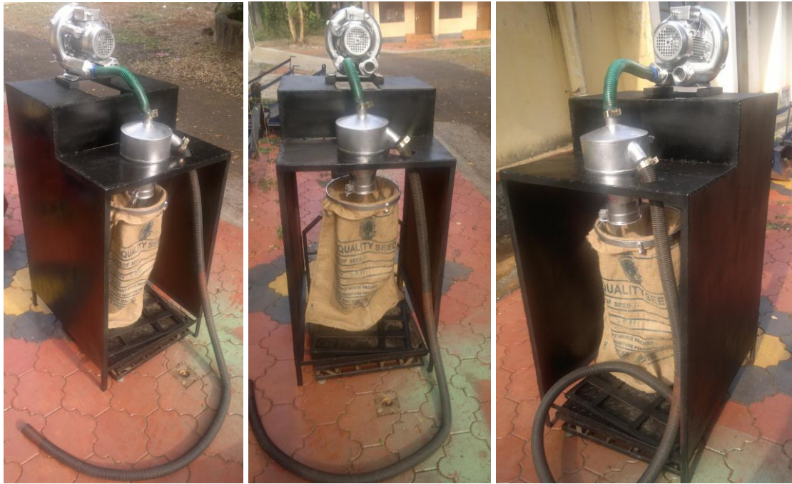
Plate 4.1 Different views of the Pneumatic Packing Machine for Paddy
