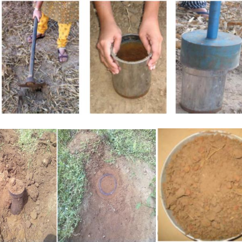
Plate 3.1 Sampling by core cutter
