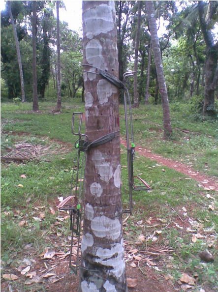
Plate 3.1 Kerala model coconut palm climbing device
