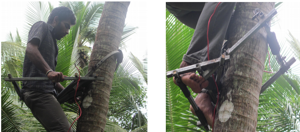
Plate 4.2 Testing with modified coconut palm climbing device
