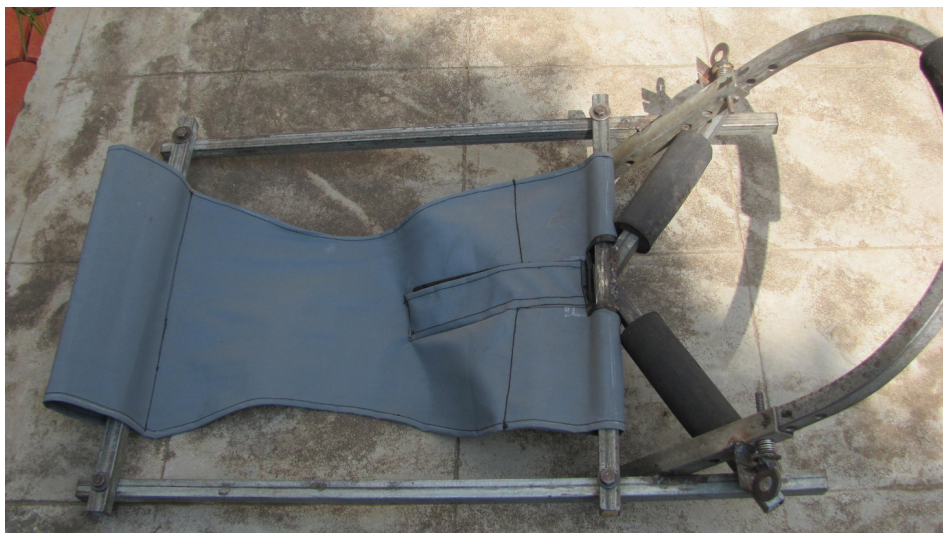
Plate 4.3 Upper frame of the modified model of coconut palm climbing device
