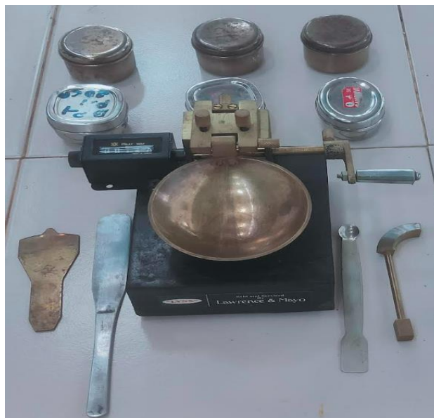
Plate 3.1 Determination of liquid limit of soil
