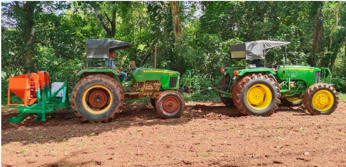
Plate 3.16 Draft measurement in field
