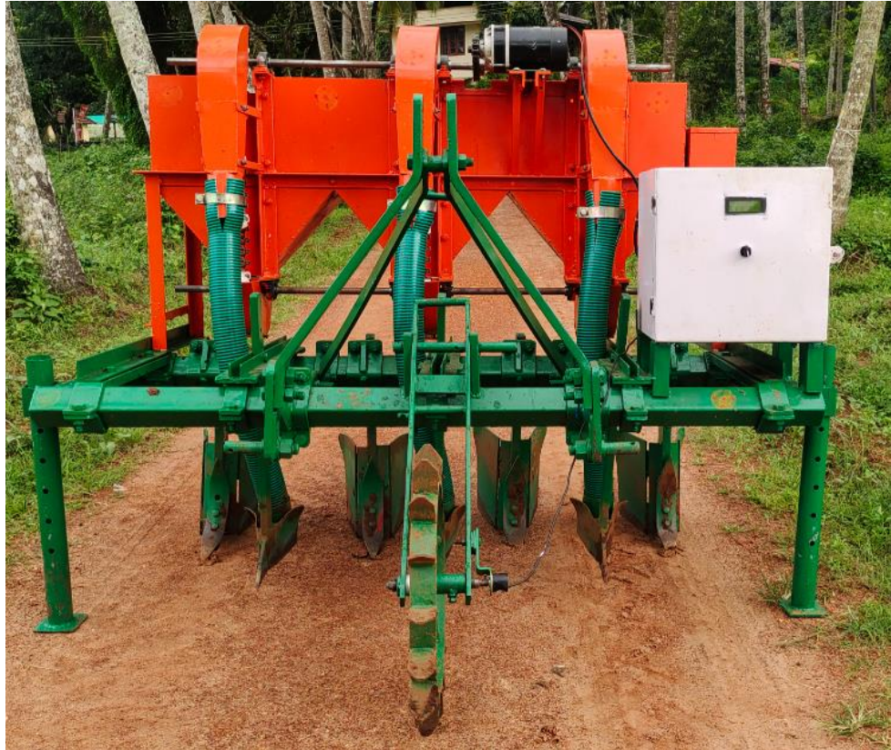
Plate 3.14 Developed sensor-based tractor drawn ginger planter
