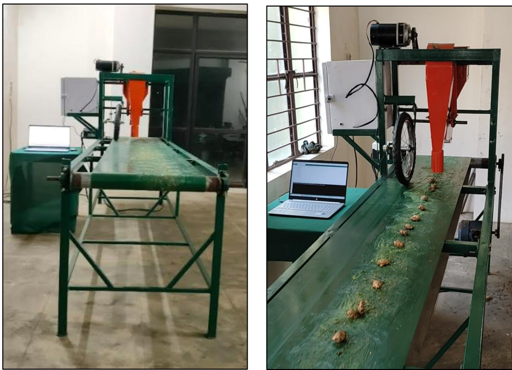
Plate 3.9 Developed laboratory set up for the sensor-based tractor drawn ginger planter
