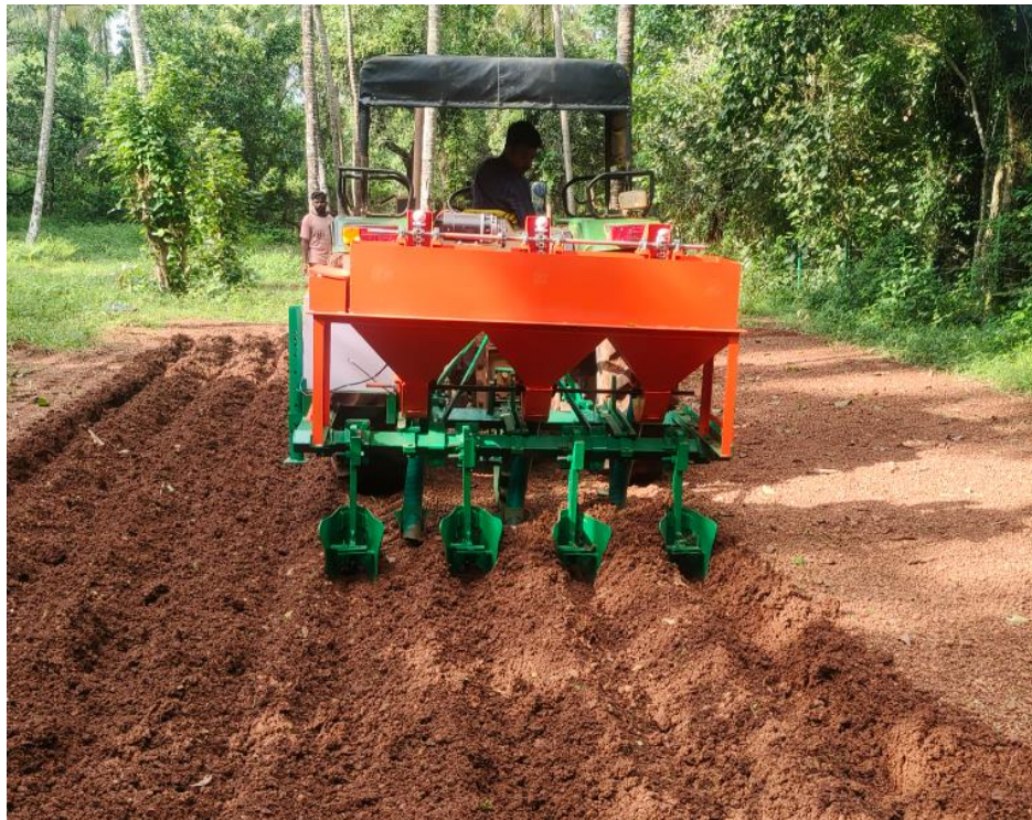
Plate 3.15 Working of a developed sensor-based tractor drawn ginger planter
