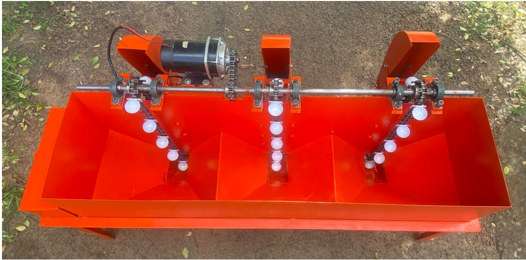
Plate 3.10 Top view of the sensor based ginger hopper
