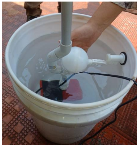
Plate 3.8 Float valve installed inside supply tank
