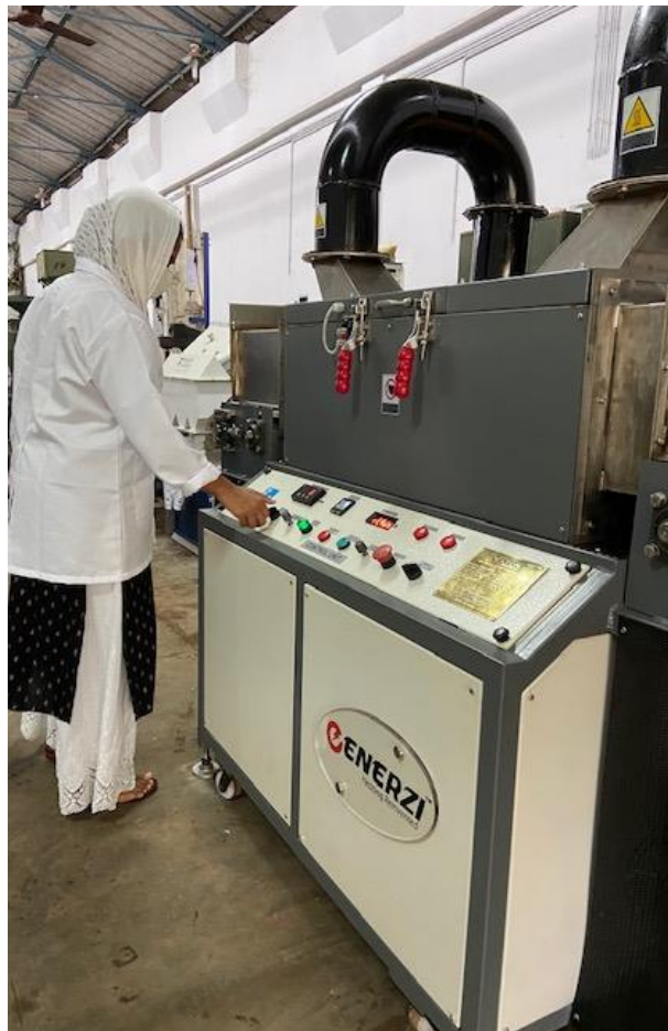
Plate 4.2 Working photograph on microwave convective dryer
