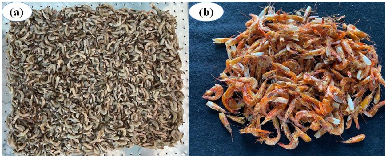
Plate 4.3 Photograph of shrimp before (a) and after drying (b) under a hot air-assisted microwave drying system
