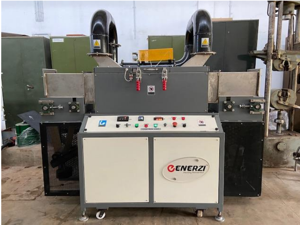
Plate 4.1 Photograph of microwave convective dryer installed at KCAET, Tavanur
