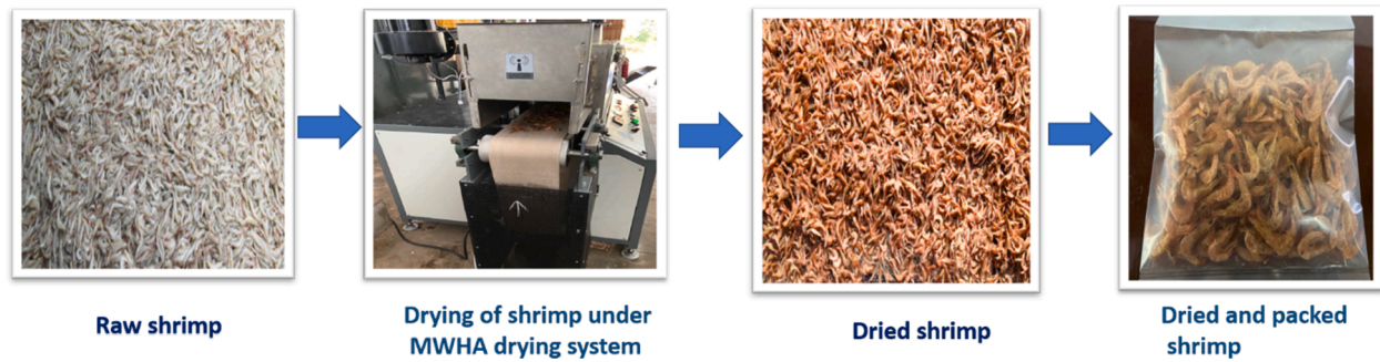
Fig. 2. Drying of shrimp under microwave drying system.
