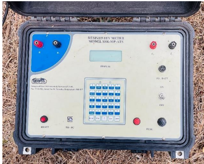
Plate 3.4 Data Acquisition unit of Electrical resistivity meter
