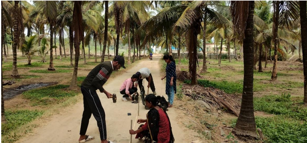
Plate 3.9 VES survey using Electrical resistivity meter
