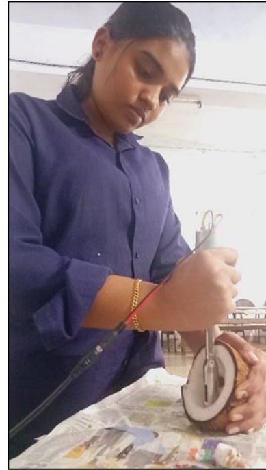
Plate. 3.5 Evaluation of coconut embryo plug scooping tool in lab
