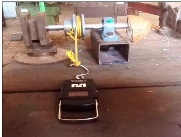
Plate. 3.2 Experimental setup for torque measurement
