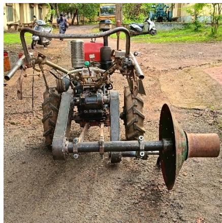
Plate 4.1 Fabricated power tiller operated ridge plastering machine
