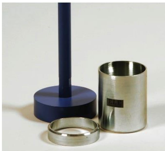
Fig 3.19 Core cutter, dolly and rammer
