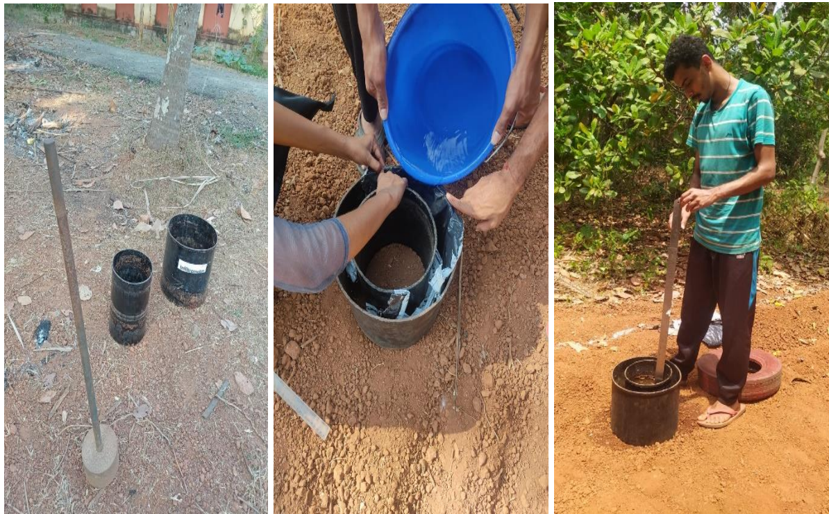
Plate 9 Determining infiltration rate by double ring infiltrometer
