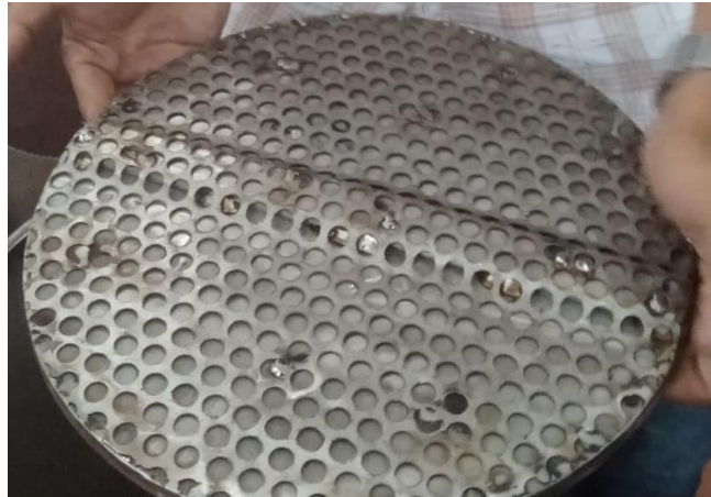
Plate 3.9 Rotating disc with perforated sheet and agitating strip
