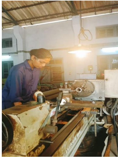
Plate 3.11 Boring of shaft
