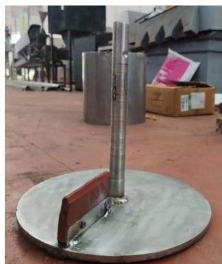
Plate 3.10 Connecting shaft welded on the rotating disc
