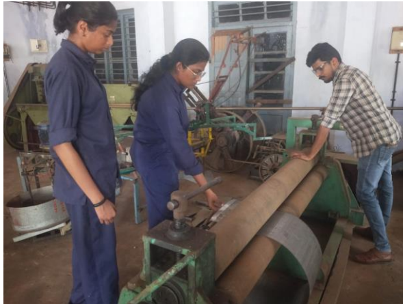
Plate 3.7 Bending of perforated sheet
