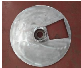
Plate 3.8 Base plate with ring and bearing and trapezoidal slit
