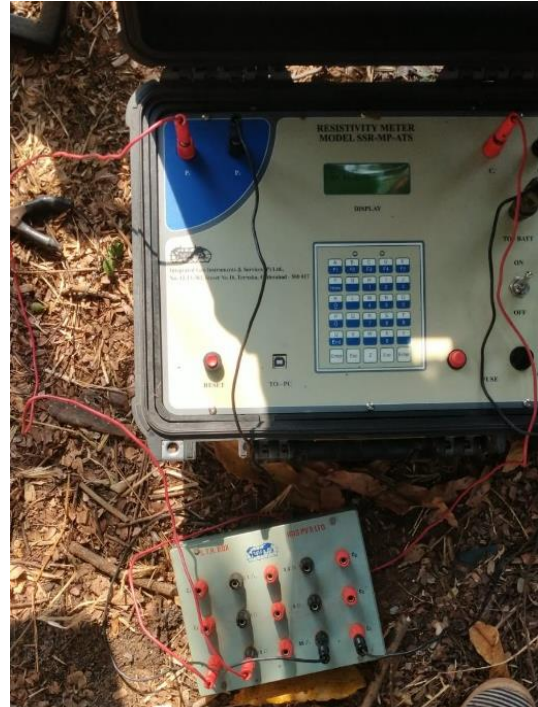
Plate 3.9 Calibration of Electrical resistivity meter
