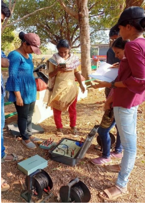
Plate 3.9 Calibration of Electrical resistivity meter
