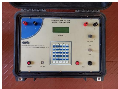
Plate 3.4 Data Acquisition unit of Electrical resistivity meter
