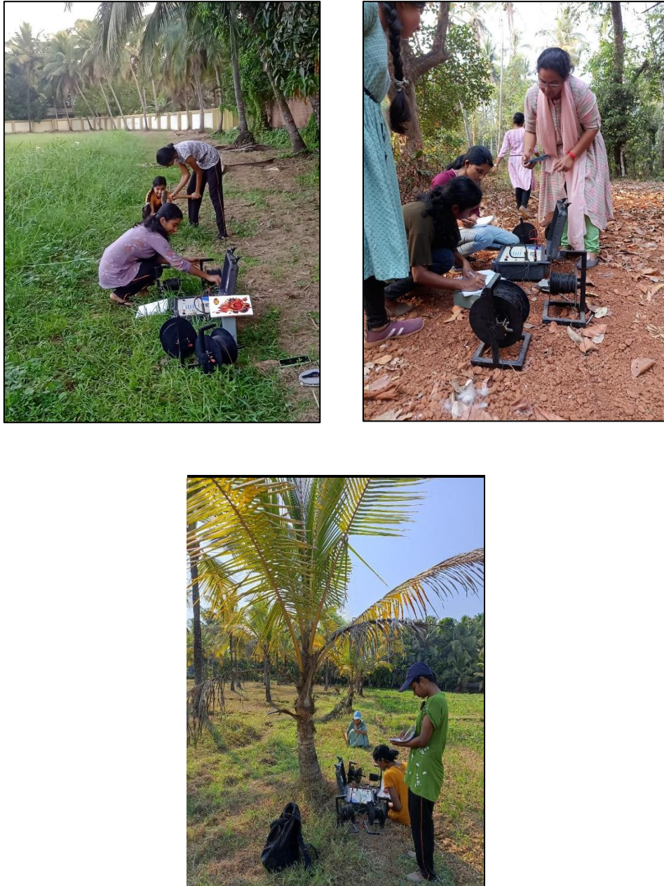
Plate 3.11 VES survey using Electrical resistivity meter
