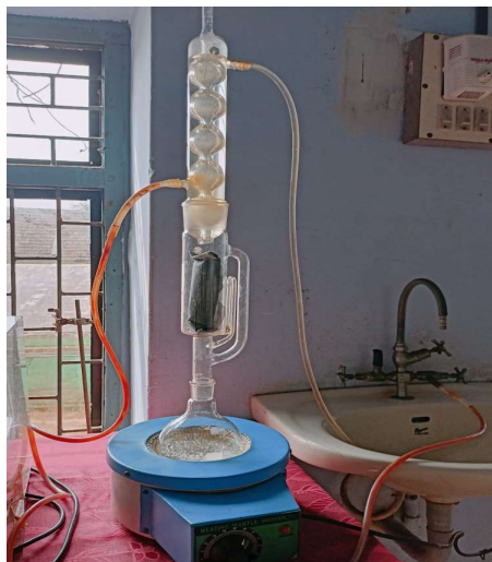
Plate 3.8. Defatting of sample with Soxhlet apparatus
