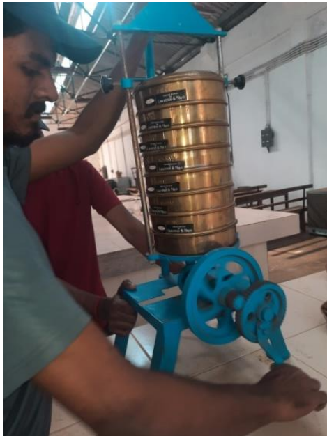
Plate 3.8 Sieve analysis using sieve shaker
