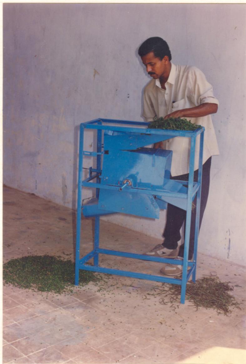
MODIFIED PEPPER THRESHER UNDER OPERATION
