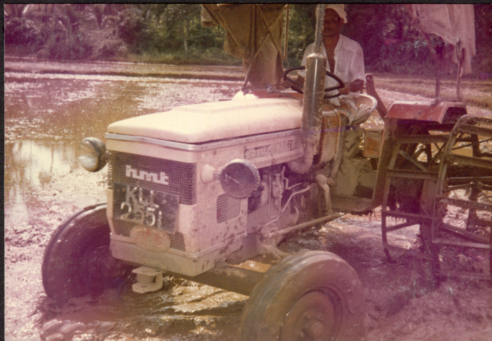
Plate No.6. Tractor with cage wheel in operation
