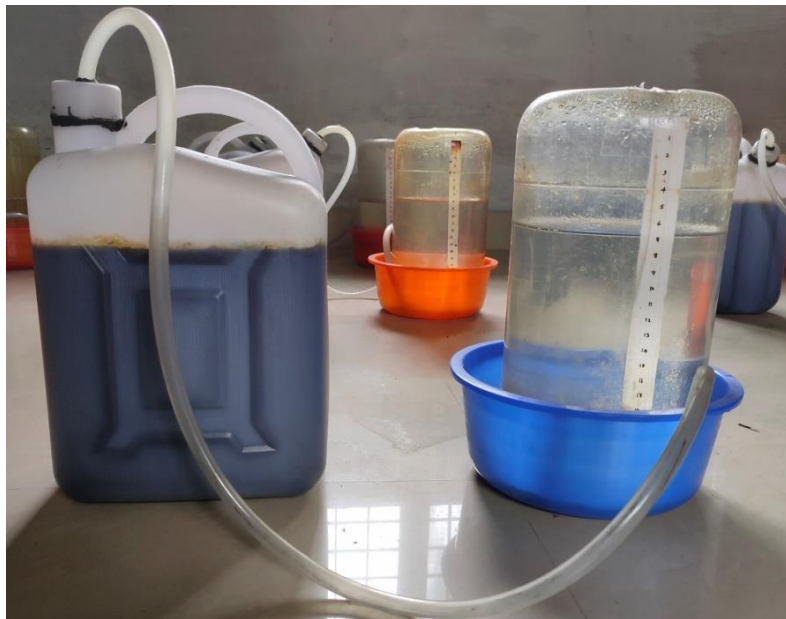
Fig. 3.5 Experimental set up for batch anaerobic digestion
