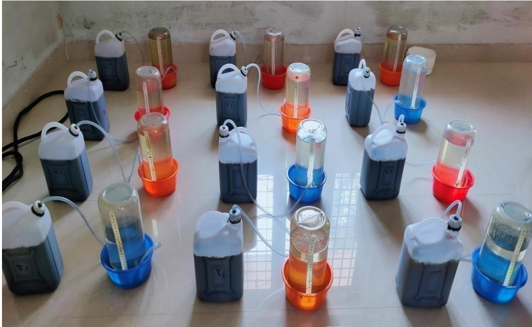
Fig. 3.6 Arrangement of experimental digesters for batch anaerobic digestion
