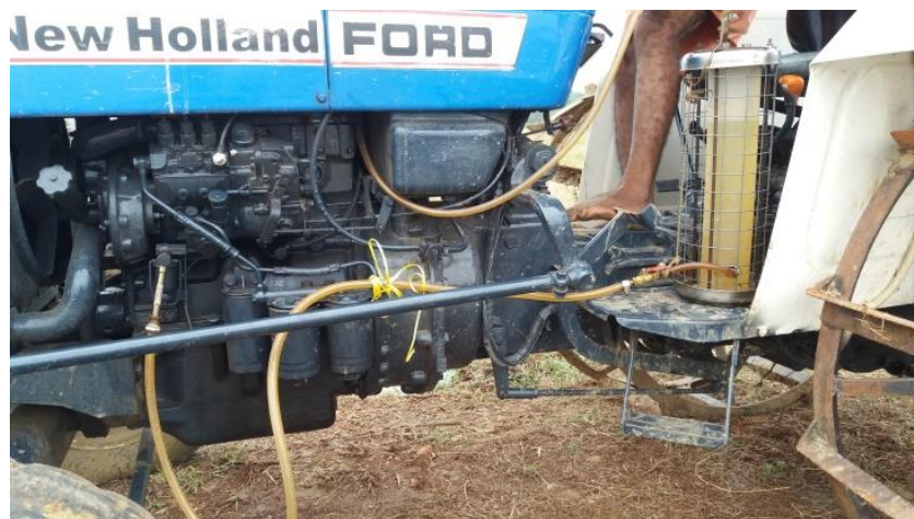
Plate 3.16 Setup for measurement of fuel consumption
