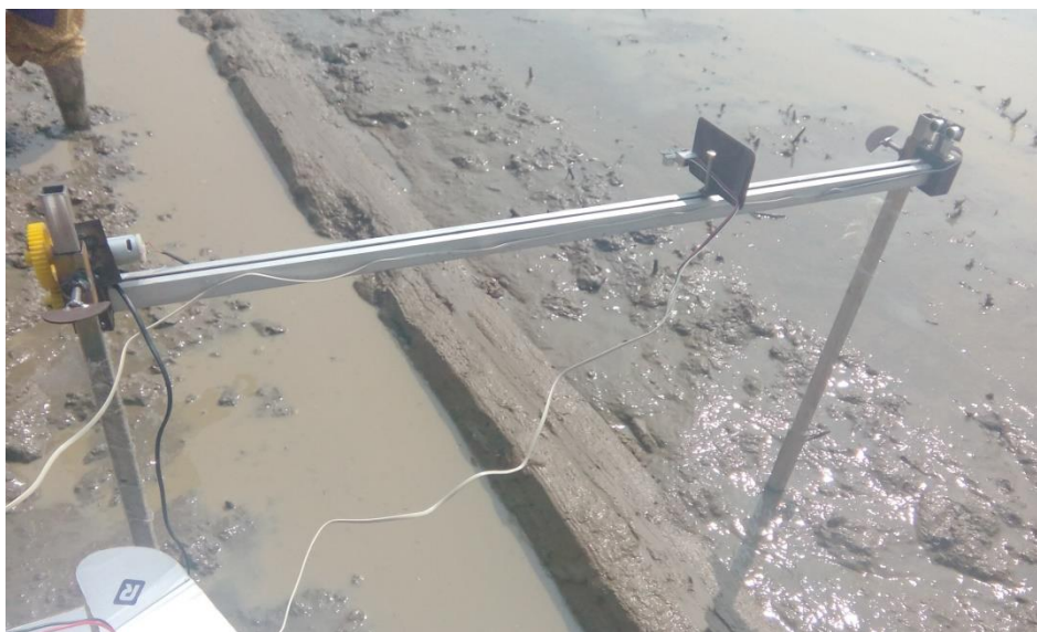
Plate 3.14 In situ measurement of the bund profile
