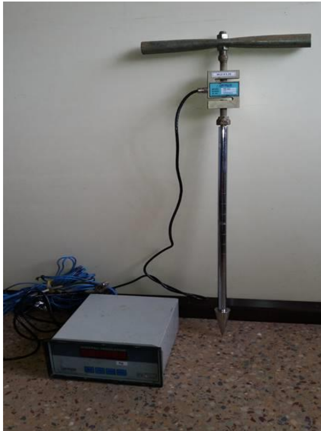
Plate 3.8 Set up for measurement of cone index
