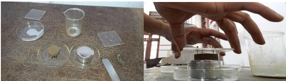
Plate 3.7 Determination of shrinkage limit
