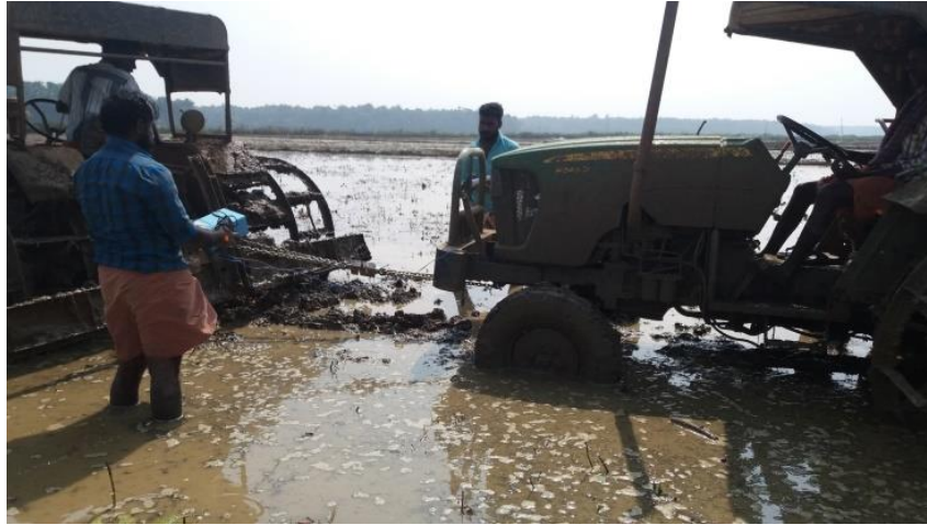
Plate 3.15 Draft measurement in field
