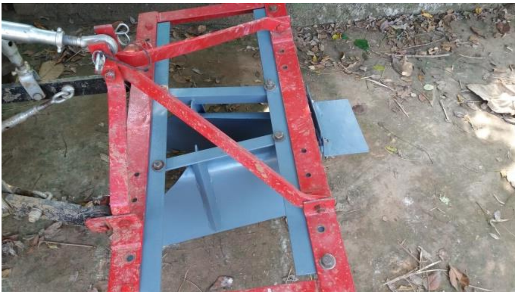
Plate 3.9 Initial model of the bund strengthening implement with rear press plate
