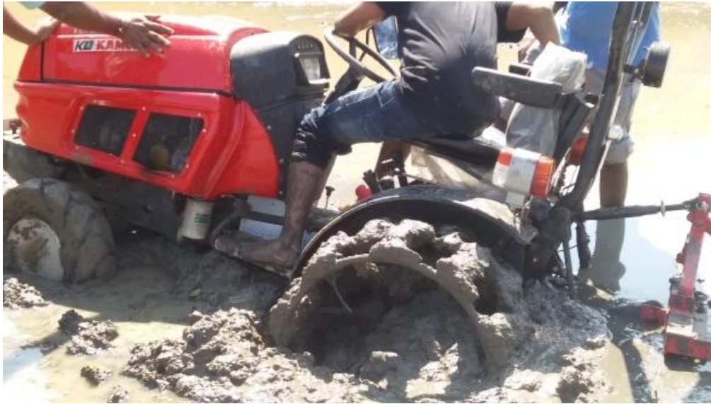
Plate 4.6 Sinking of KAMCO TeraTrac tractor at Ponnani kole
