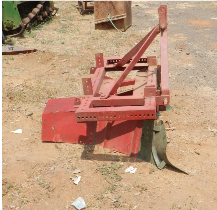
Plate 4.9 (b) Bund strengthening implement – Model BF3 – side view
