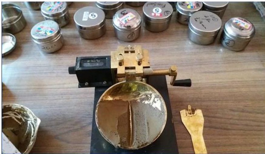
Plate 3.5 Determination of liquid limit
