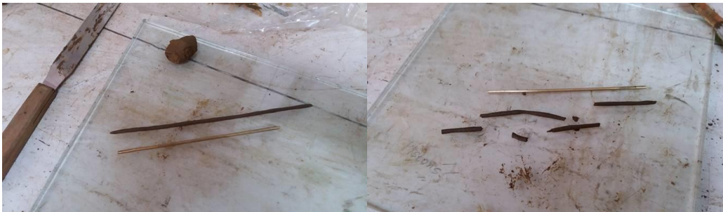
Plate 3.6 Determination of plastic limit
