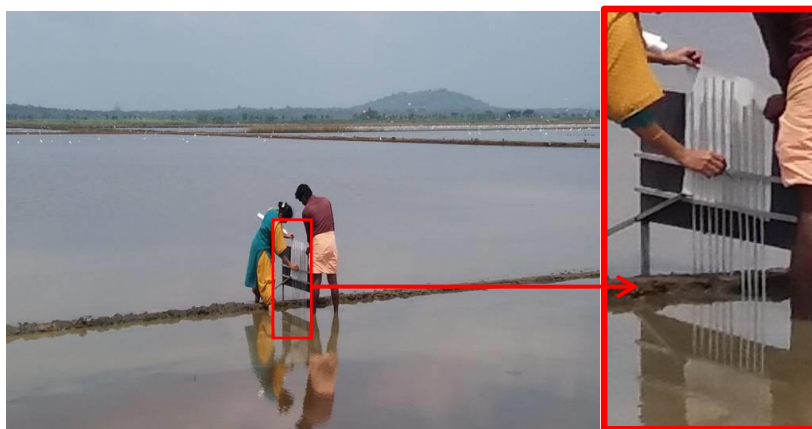
Plate 3.12 Profile measurement using pin type profilemeter
