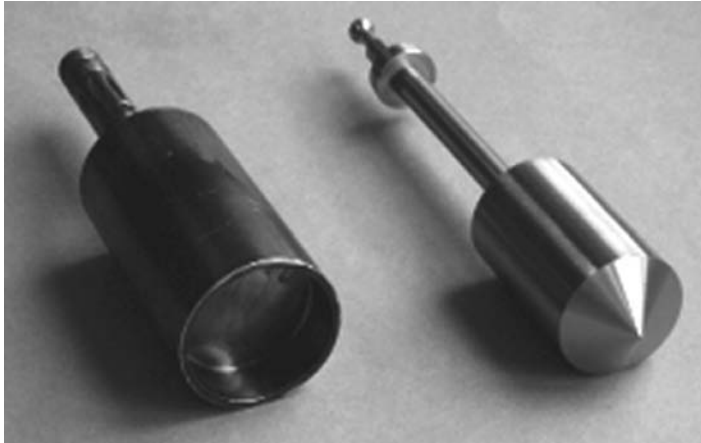
Figure 10.11 Bob types for concentric cylinder viscometer.
