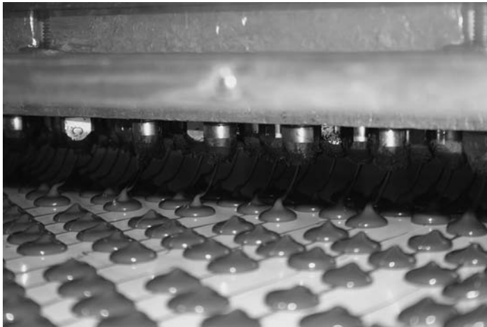
Figure 14.15 Drop moulding production plant. See Plate 11 for the colour image.
