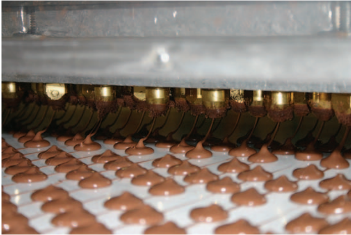
Plate 11 Drop moulding production plant.
