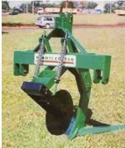
Plate 2.8. Cassava Harvester Model P900(Ospina et al. , 2002)
