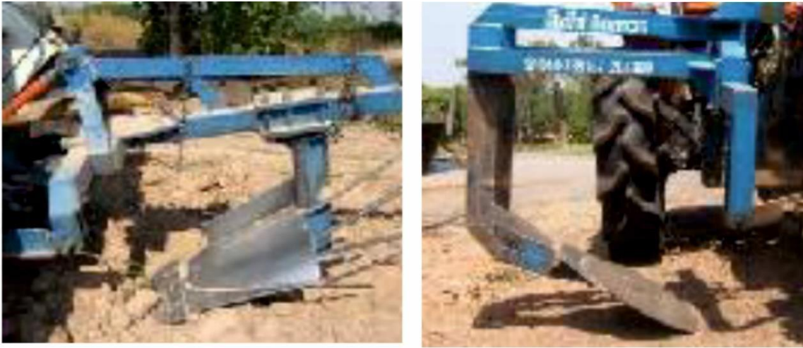
Plate 2.6. Curve Blade Harvester (Chalachai et al. , 2013)
