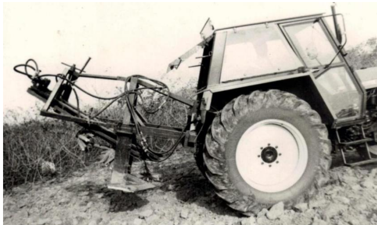
Plate 2.7. Mechanical Cassava Harvester designed by Leipzig University
