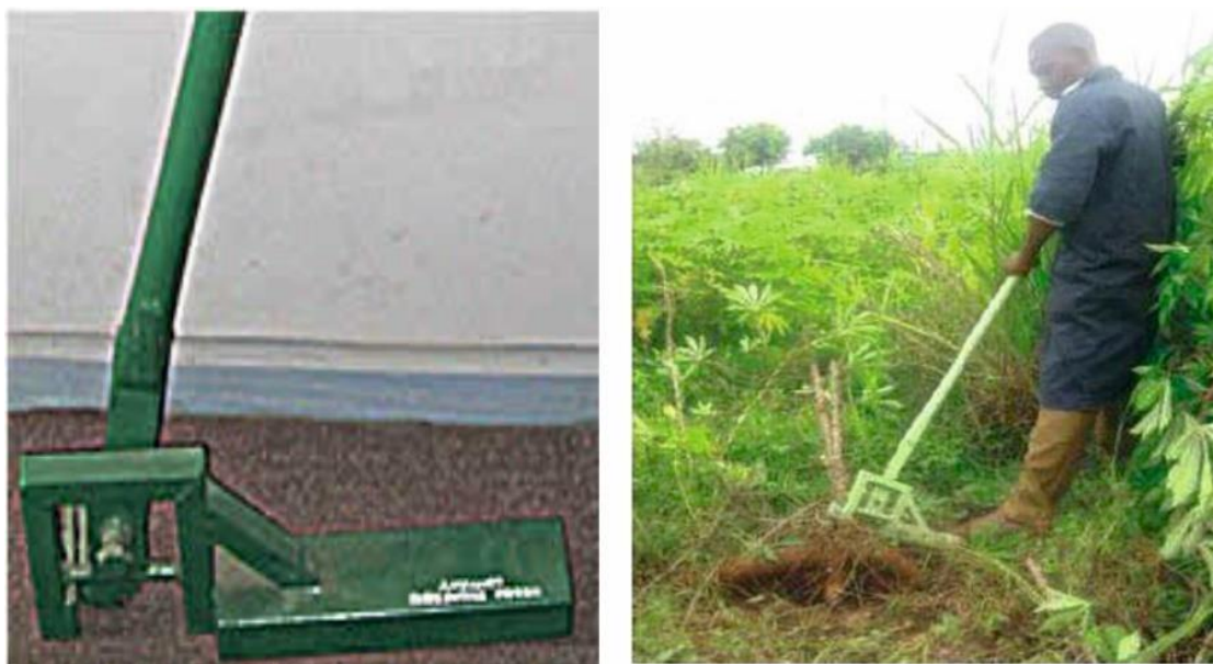
Plate 2.4. Cassava harvester designed by NCAM (Amponsah et al. , 2018)
