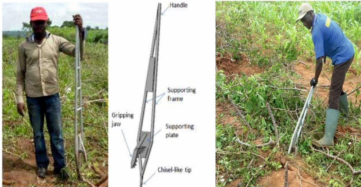
Plate 2.3. Cassava Harvester designed by CRI (Shadrack et al. , 2017)
