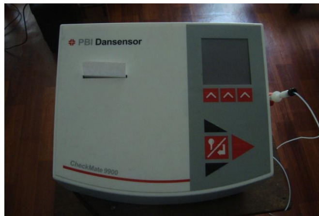
Plate 3.3 Experimental setup for gas composition determination (Check Mate2)
