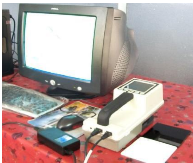
Plate 3.2 Experimental set up of Hunter lab colour flex meter
