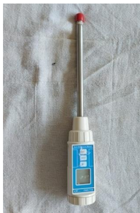
Plate 3.9 Soil moisture meter
