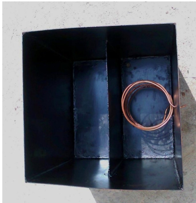
Plate 1. Sectional view of Humidification De-Humidification Chamber
