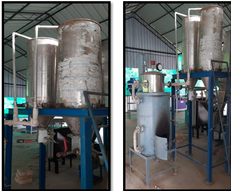
Plate 3.2 Soaking cum steaming chamber
