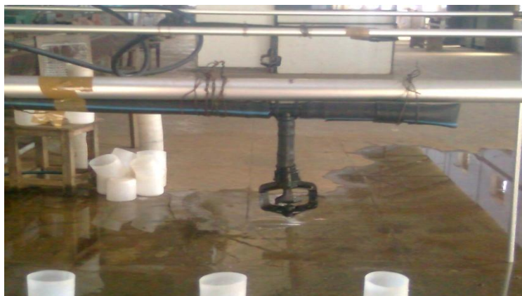
Plate 2: Rainfall simulation using microsprinklers
