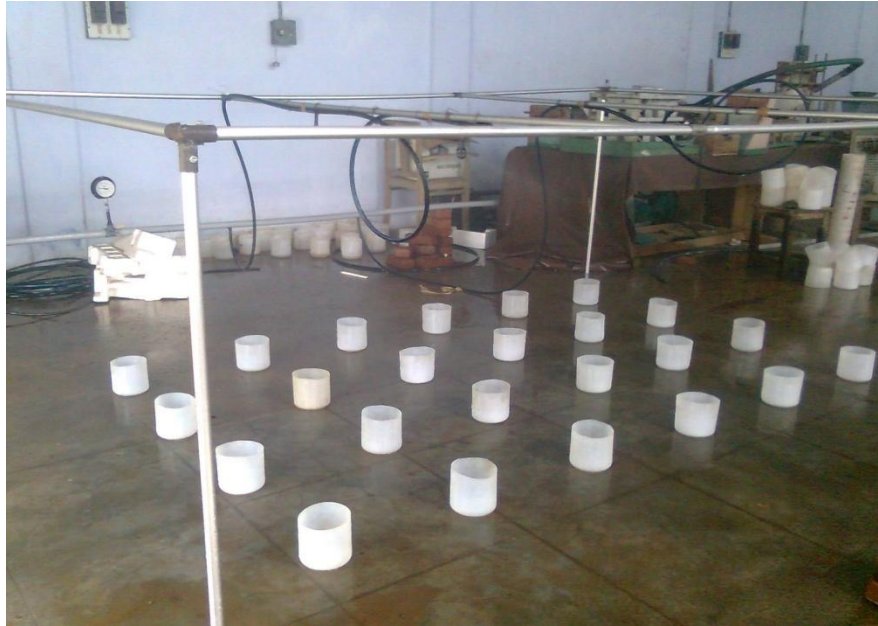
Plate 5: Rainfall simulator testing for intensity and uniformity in the lab
