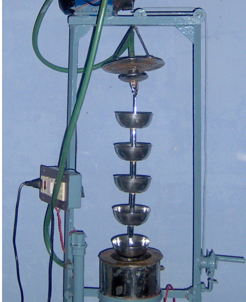
Plate 3.6. Cup assembly with wire and pulley arrangement
