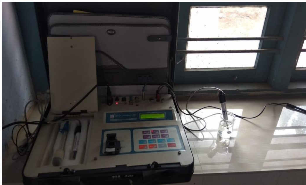
Fig 3.4 Salinity analysis using water analyzer
