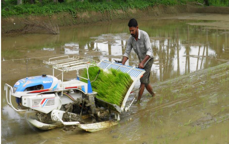
**Plate 3.15 Mechanical transplanting by male operator**
