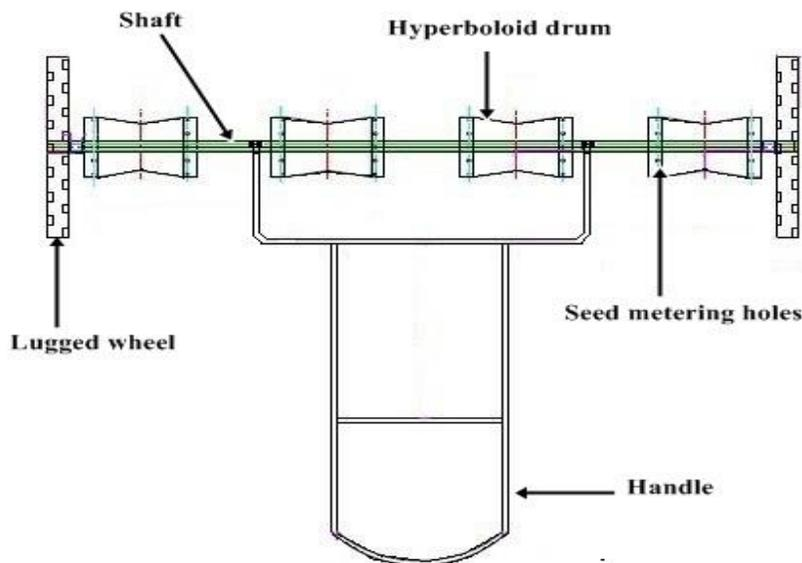
**Fig 3.1 Schematic of Direct paddy seeder**
