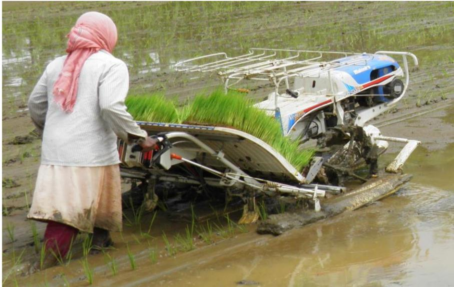
**Plate 3.16 Mechanical transplanting by female operator**
