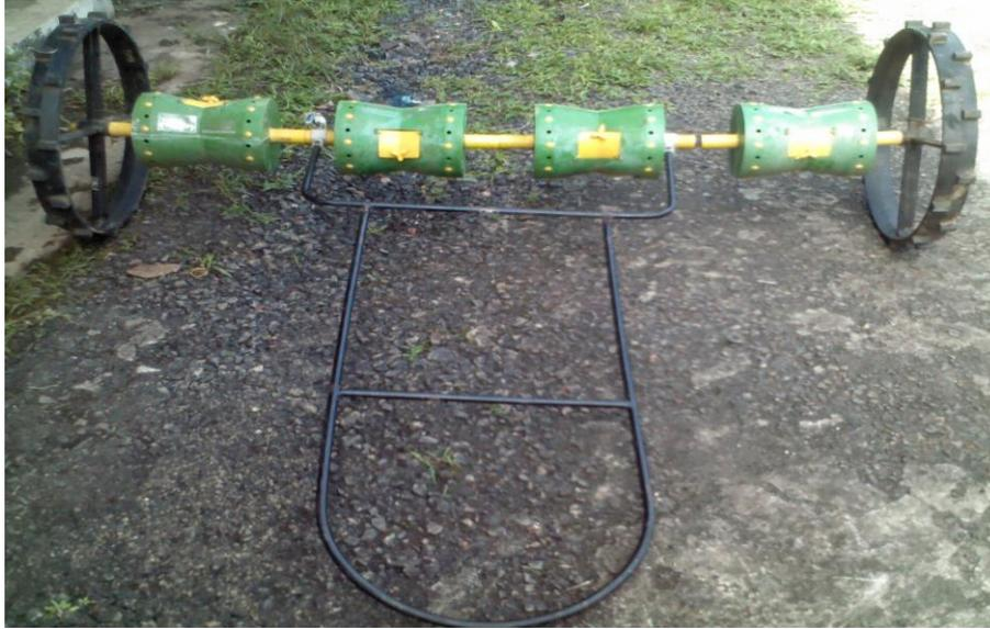
**Plate 3.9 Direct paddy seeder (Drum seeder)**
