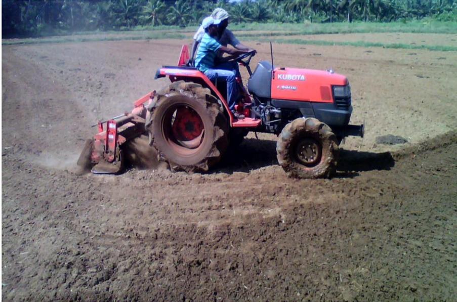
**Plate 3.6 Ploughing by tractor mounted rotavator**
