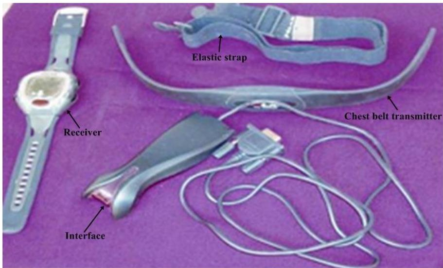
**Plate 3.19 Polar S 810 computerized heart rate monitor**
