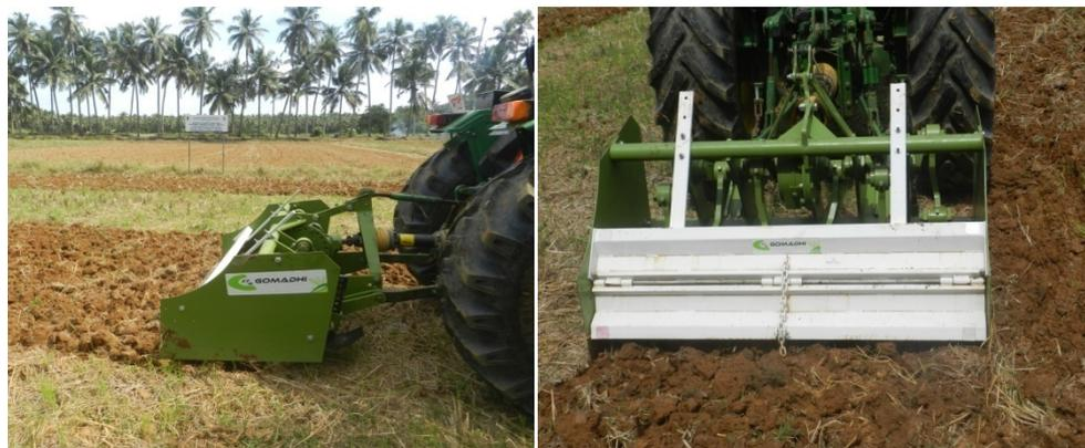
Fig. 3.9 Spading machine operation
