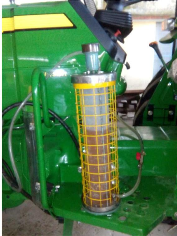
Fig. 3.6 Fuel consumption measuring setup
