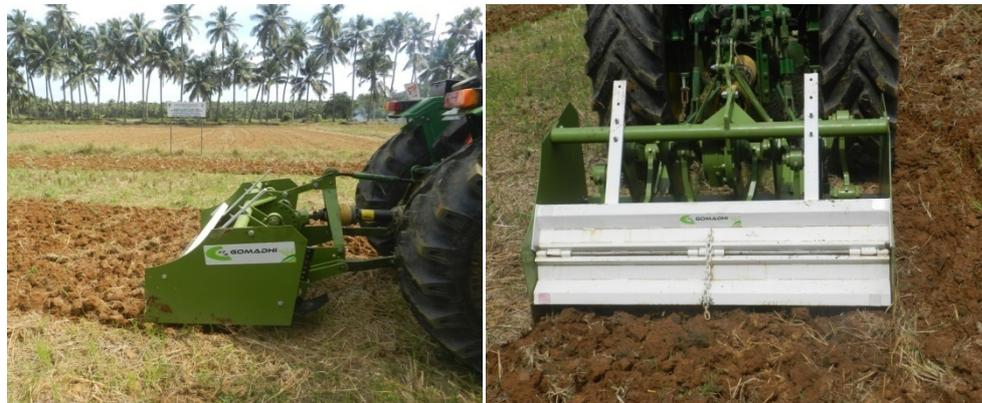
Fig. 3.9 Spading machine operation
