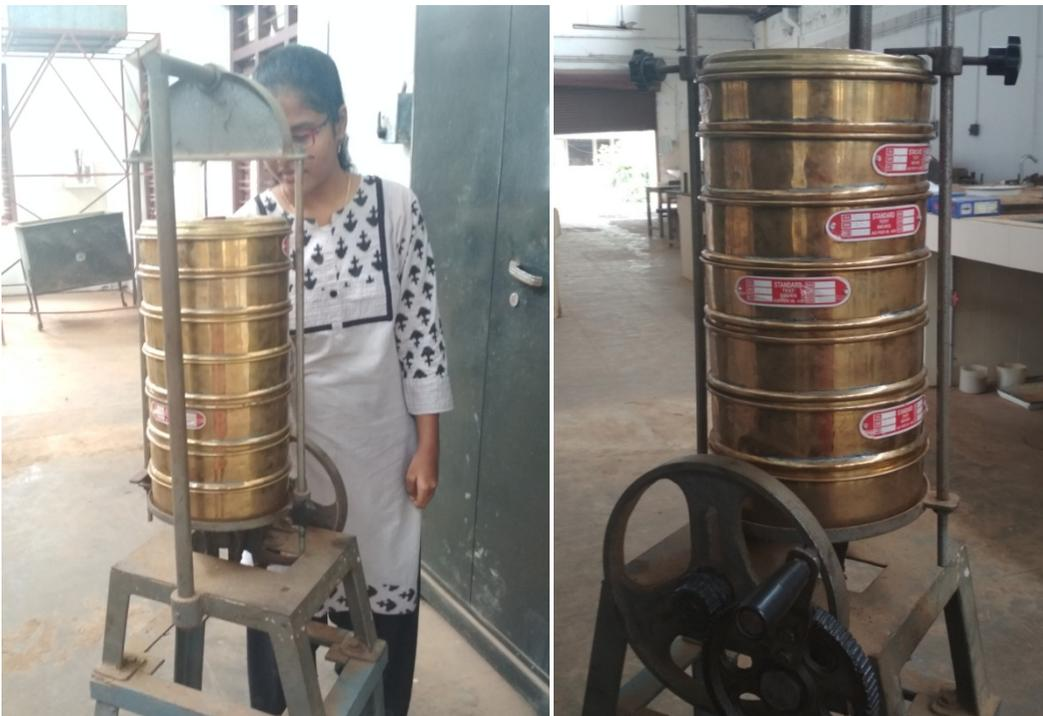
Fig. 3.5 Determination of MMD using sieve analysis
