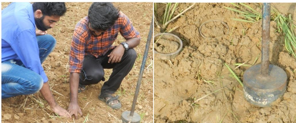
Fig. 3.2 Determination of soil bulk density by core cutter method
