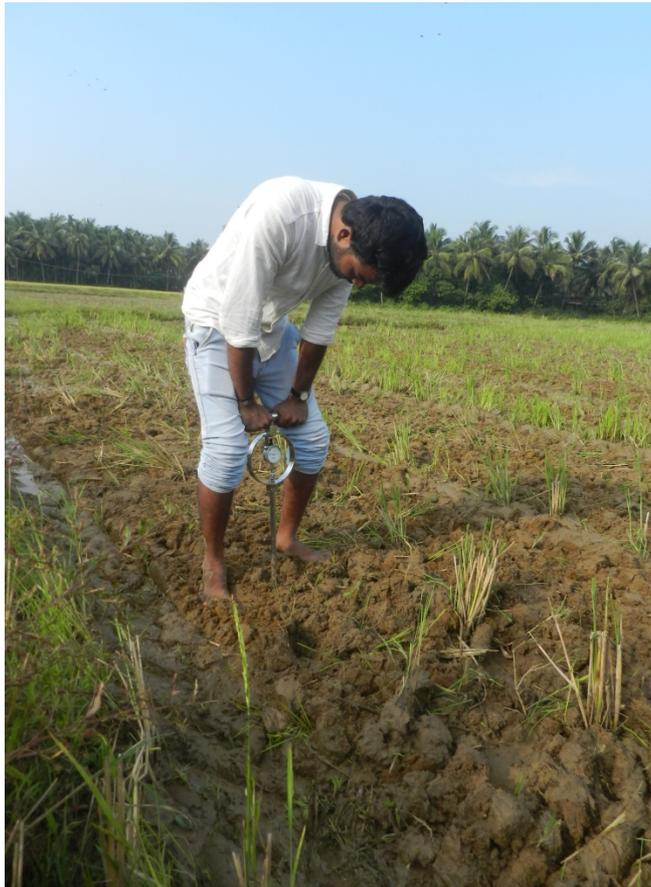
Fig. 3.3 Measurement of penetration resistance using cone penetrometer
