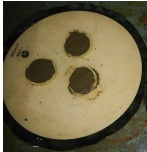
Plate 18. Ceramic plate (1 bar)
