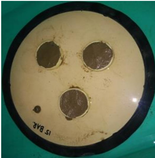
Plate 17. Ceramic Plate (15 bar)
