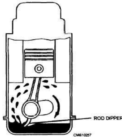
Fig,Splash lubrication system
