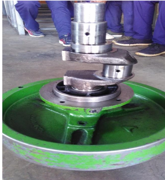
Fig. Crank shaft with flywheel
