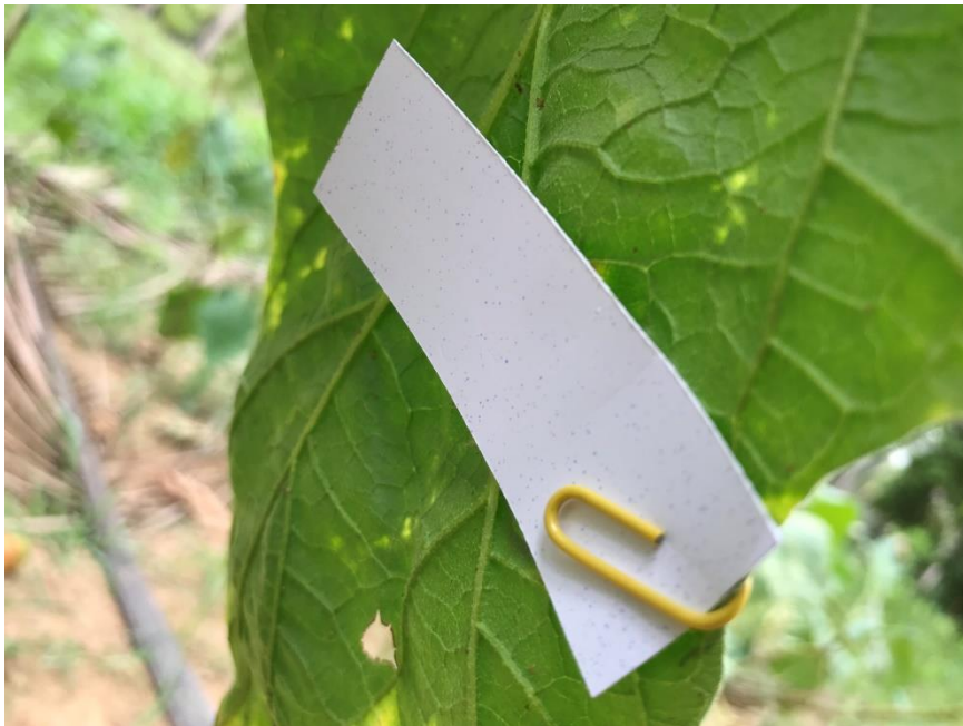
Fig. 4.20 Abaxial deposition by electrostatic spraying
