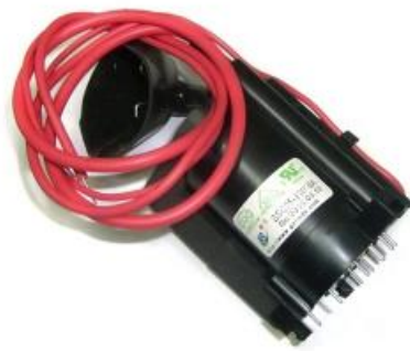
Fig. 4.1 Line Output Transformer (LOPT) or flyback transformer
