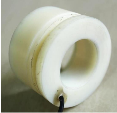
Fig. 4.5 HVDC electrostatic induction charging electrode assembly
