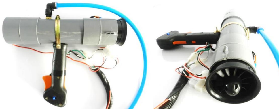
Fig. 4.13 Developed air assisted electrostatic spray gun
