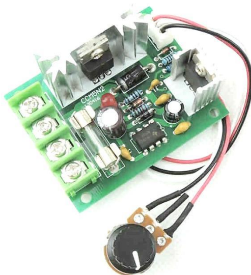
Fig. 4.4 Pulse Width Modulator (PWM)
