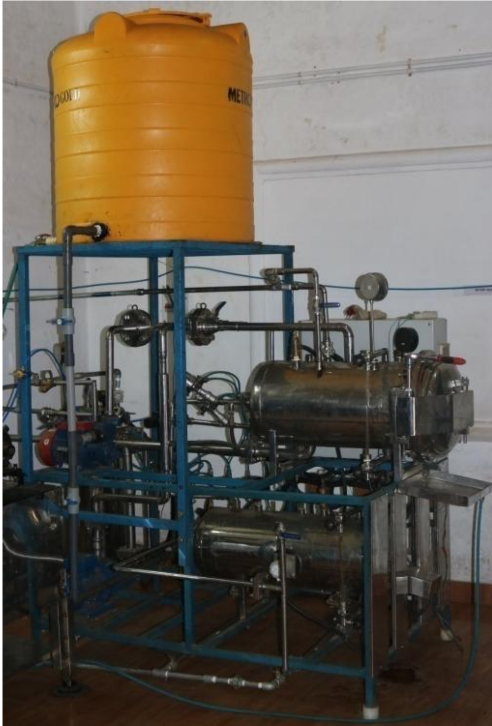
Plate 3.1a Steam-air semiautomatic retort
