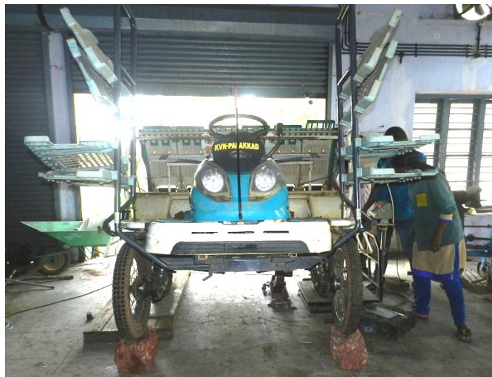
Figure 3.5 Experimental setup for finding centre of gravity
