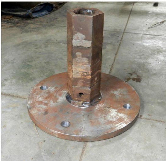
Figure 4.6 Fabricated rear wheel hub attachment
