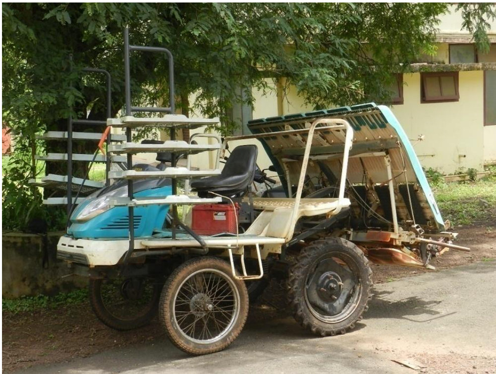
Figure 4.8 Transplanter with pneumatic wheels
