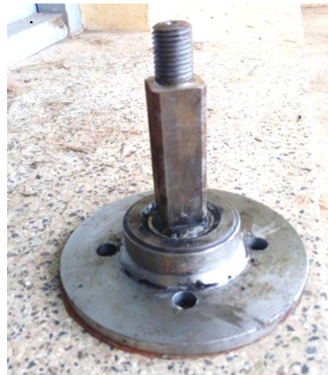
Figure 4.7 Fabricated front wheel hub attachment
