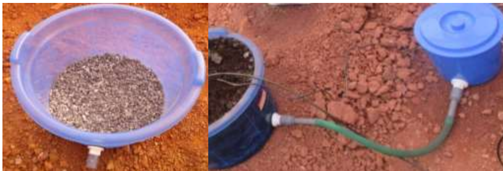
Plate 3.5 Non-weighing Mini lysimeter with drainage system
