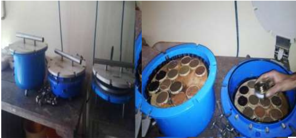
Plate 3.2 Soil moisture constants by Pressure plate apparatus
