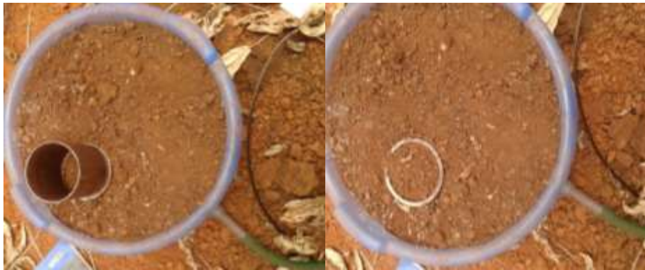
Plate 3.1 Determination of Bulk density by Core cutter
