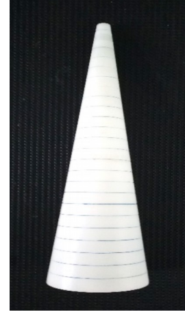
Plate 3.6 Conical device for measuring internal grip diameter
