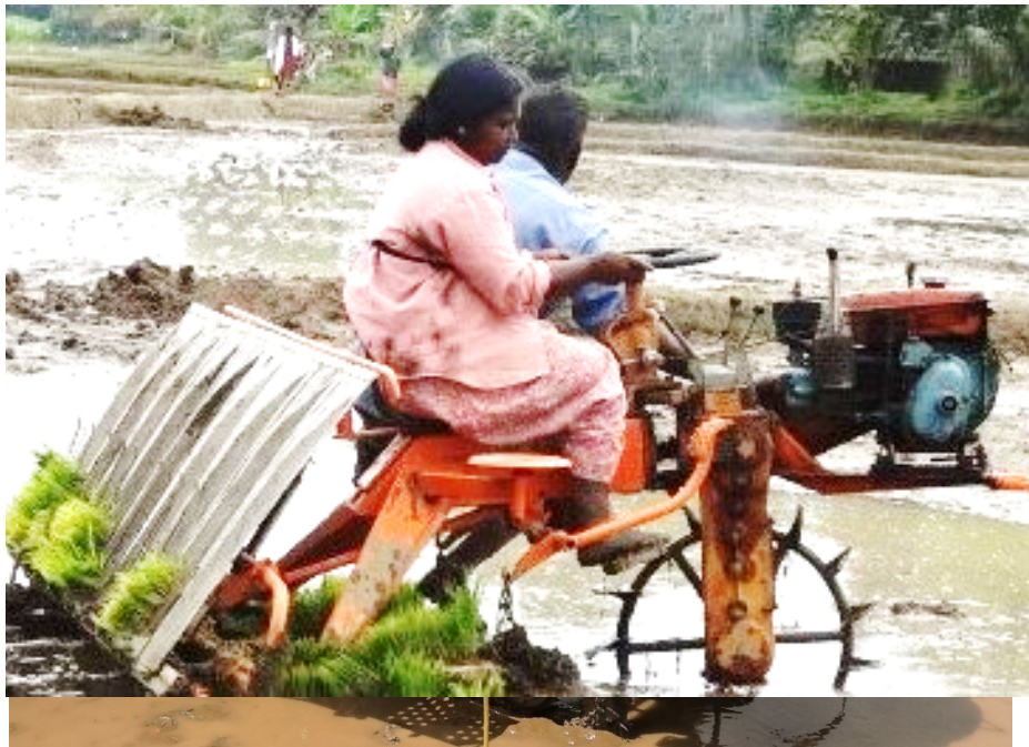
Plate 3.19. Sitting posture adopted by operator in Yanmar 8 row riding type self propelled rice transplanter
