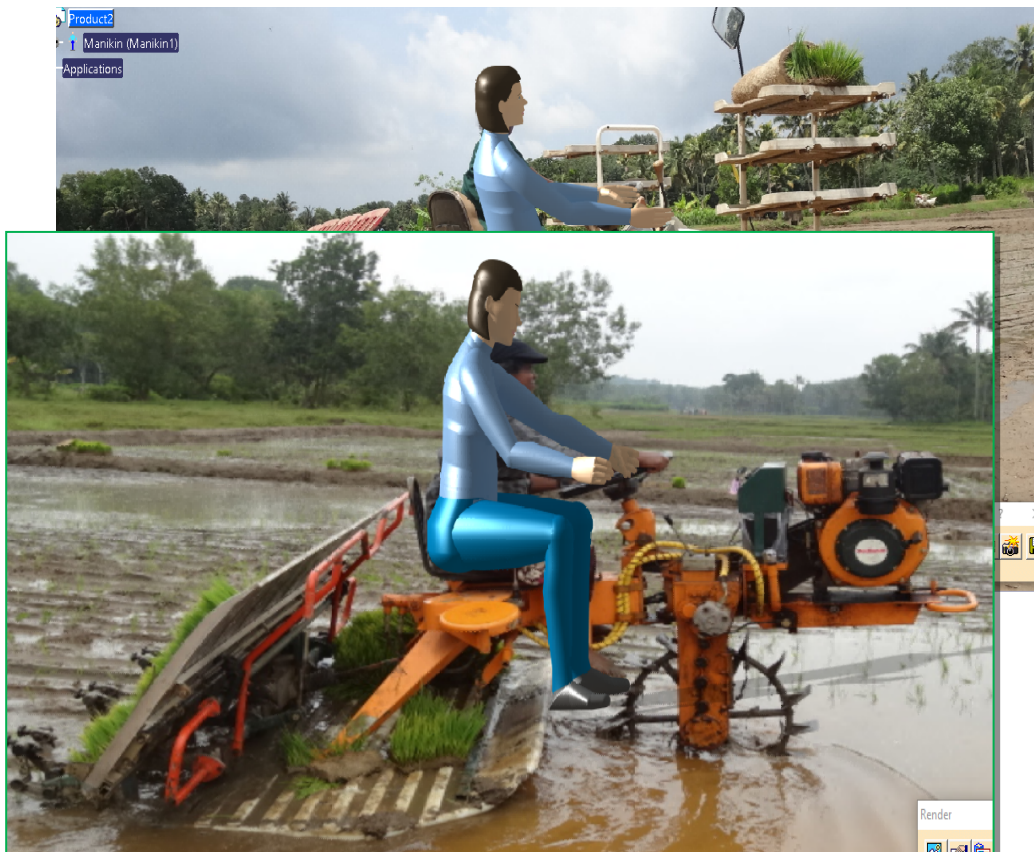
Plate 4.3. Human model posture attained by an operator in Yanmar rice transplanter (posture 3)
