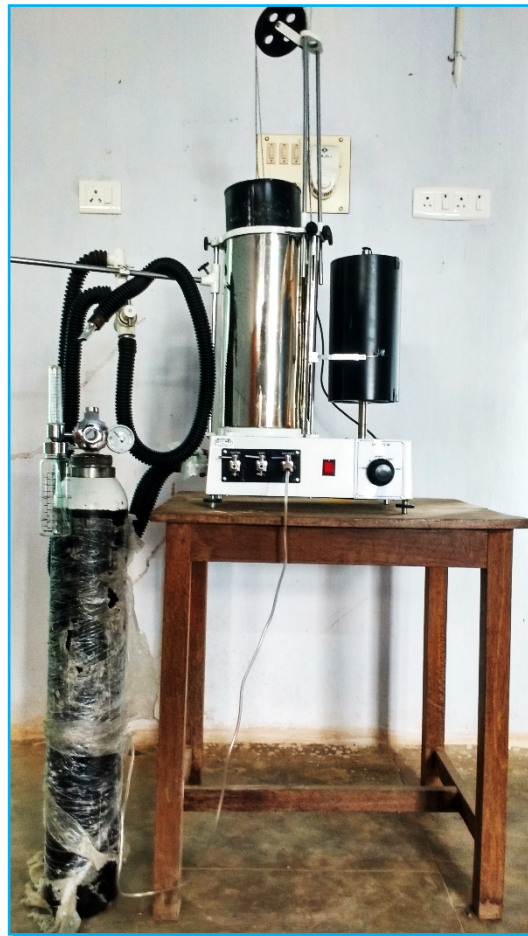
Plate 3.11. Benedict- Roth Recording Spirometer
