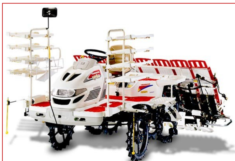
Plate 3.1. Yanmar 8 row self-propelled riding type rice transplanter
