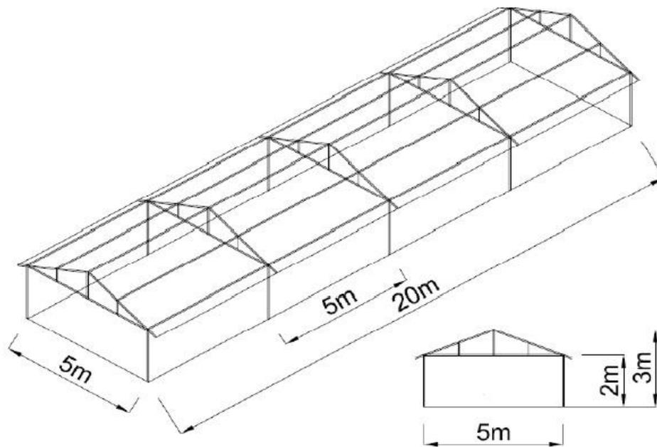
**Fig 3.2 Schematic diagram of rainshelter**
