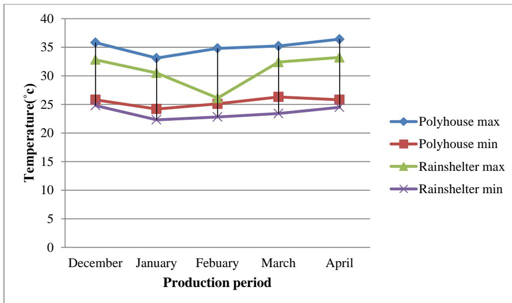
**Fig 4.2 Maximum and minimum temperature variation inside polyhouse and rainshelter at 12.30 PM**
