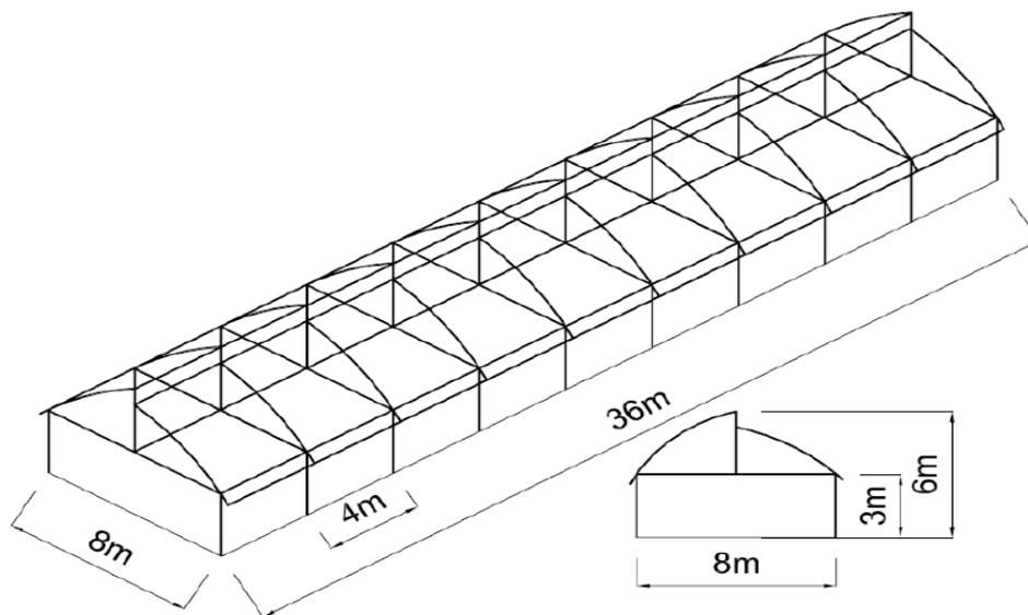
**Fig 3.1 Schematic diagram of naturally ventilated polyhouse**
