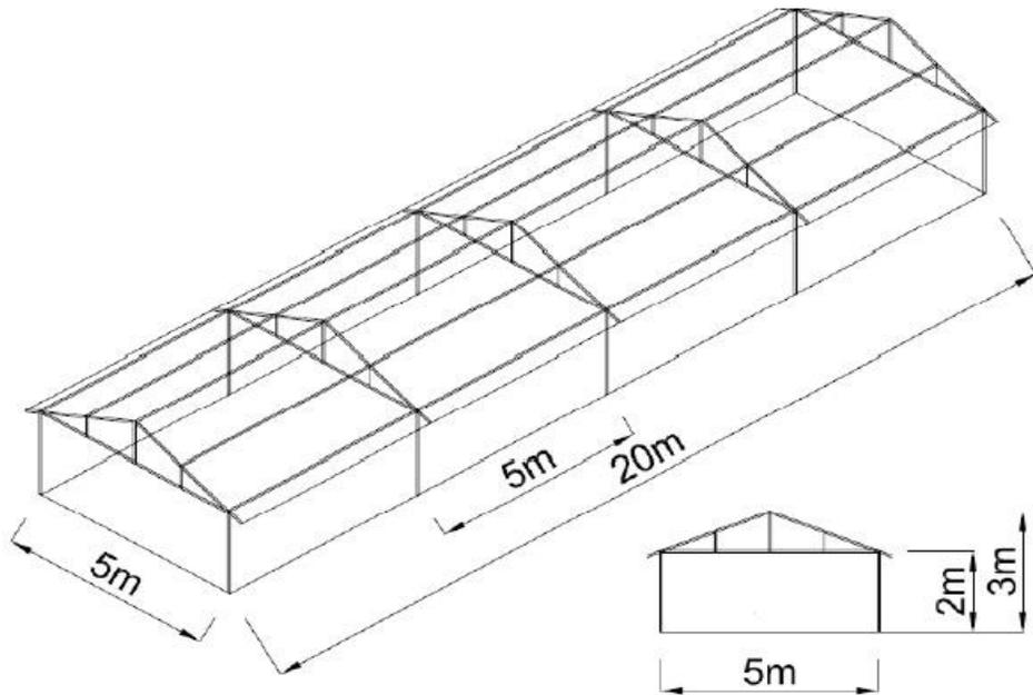
**Fig 3.2 Schematic diagram of rainshelter**
