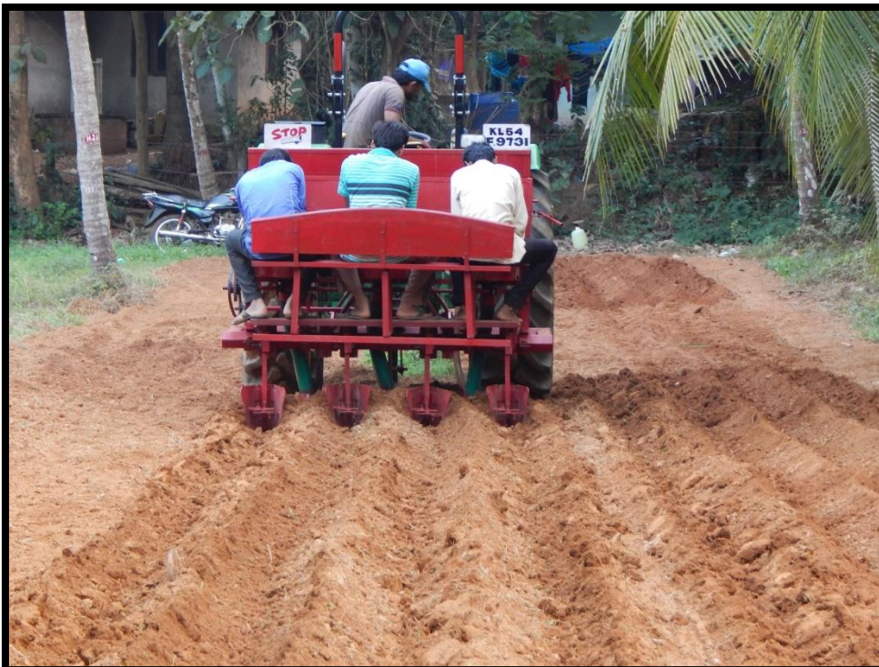
Plate 3.2 Working of developed rhizome planter in field
