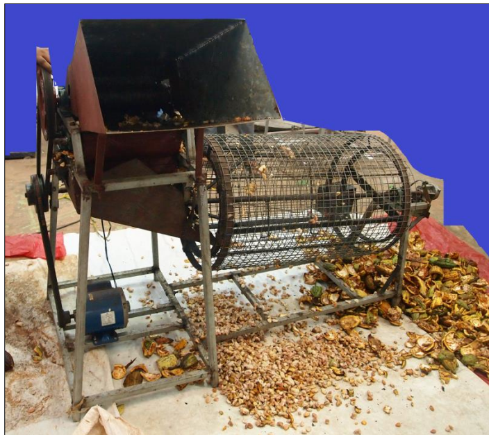
Plate 4.2. Performance evaluation of cocoa pod breaker
