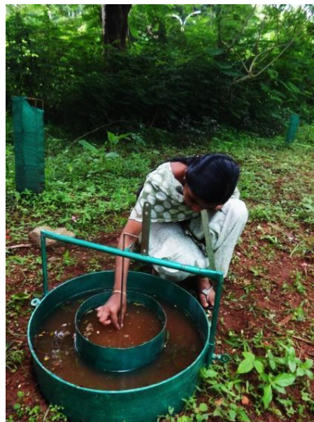
Plate 3.1 Determination of infiltration rate
