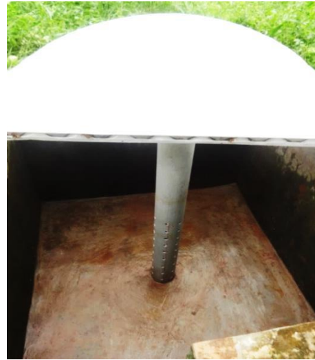
Plate 3.6 (A) Drilling holes in the pipe Plate 3.6 (B) View of holes made in the pipe
