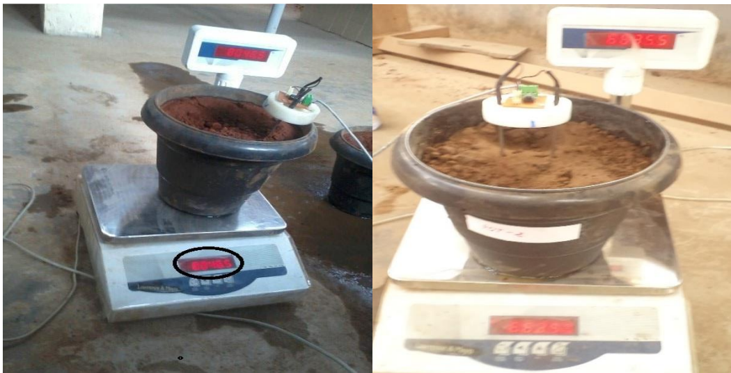
Plate 3.6 Determination of soil moisture content by weighing machine
