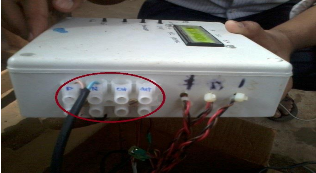
Plate 3.7 AC (230 Volts) input and output connecting terminals
