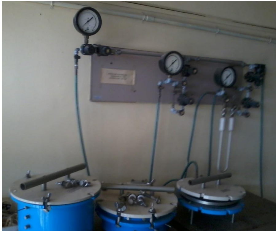
Plate 3.4 Pressure plate and membrane apparatus
