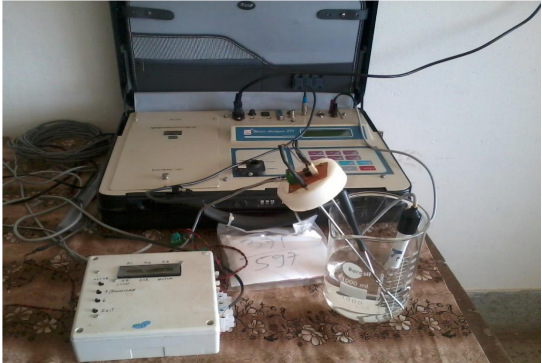
Plate 3.3 Calibration of moisture sensor in salt solution
