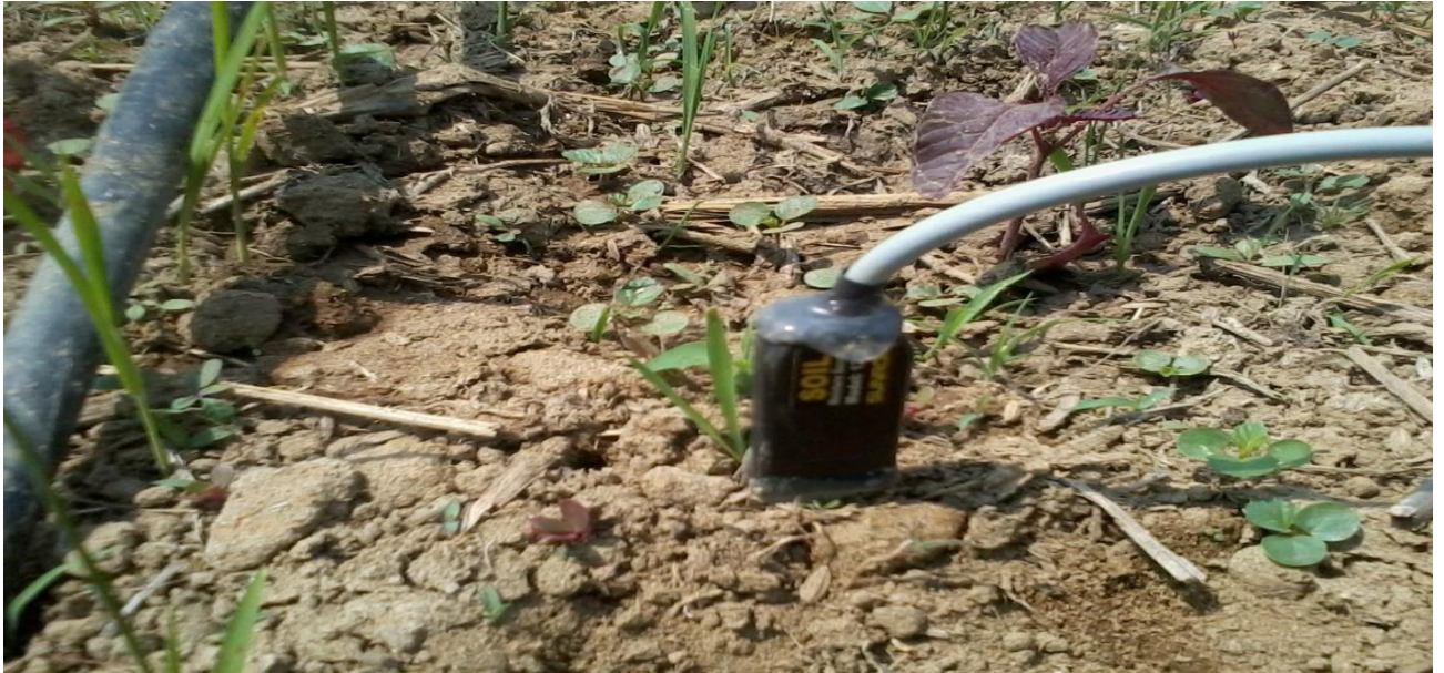
Plate 4.2 Field evaluation capacitor sensor in amrnthus crop
