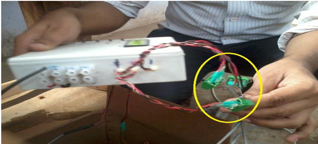
Plate 3.8 Terminal for connecting soil moisture sensors
