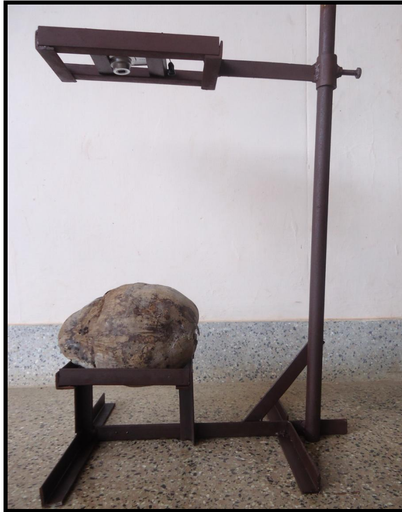
Plate 3.1 Experimental setup for taking photograph for image analysis
