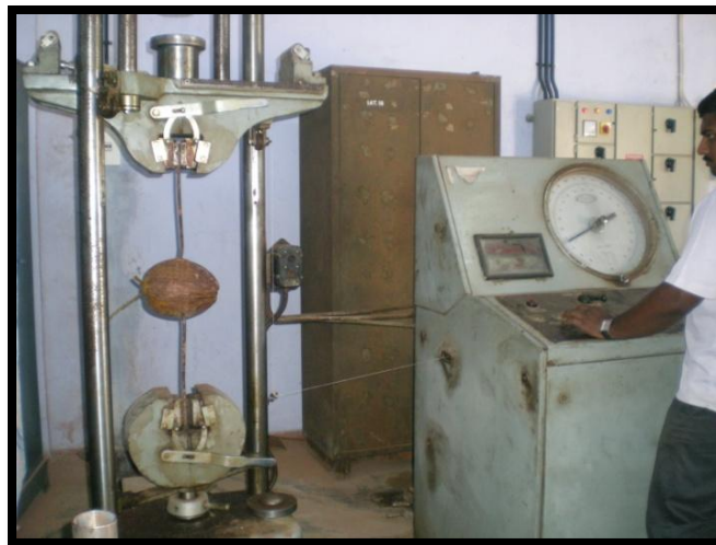
Plate 3.2 Experimental set up for determining husk separating force
