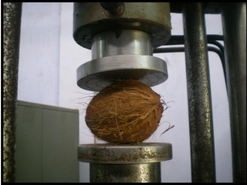
Plate 3.3 Experimental set up for determining shell breaking force
