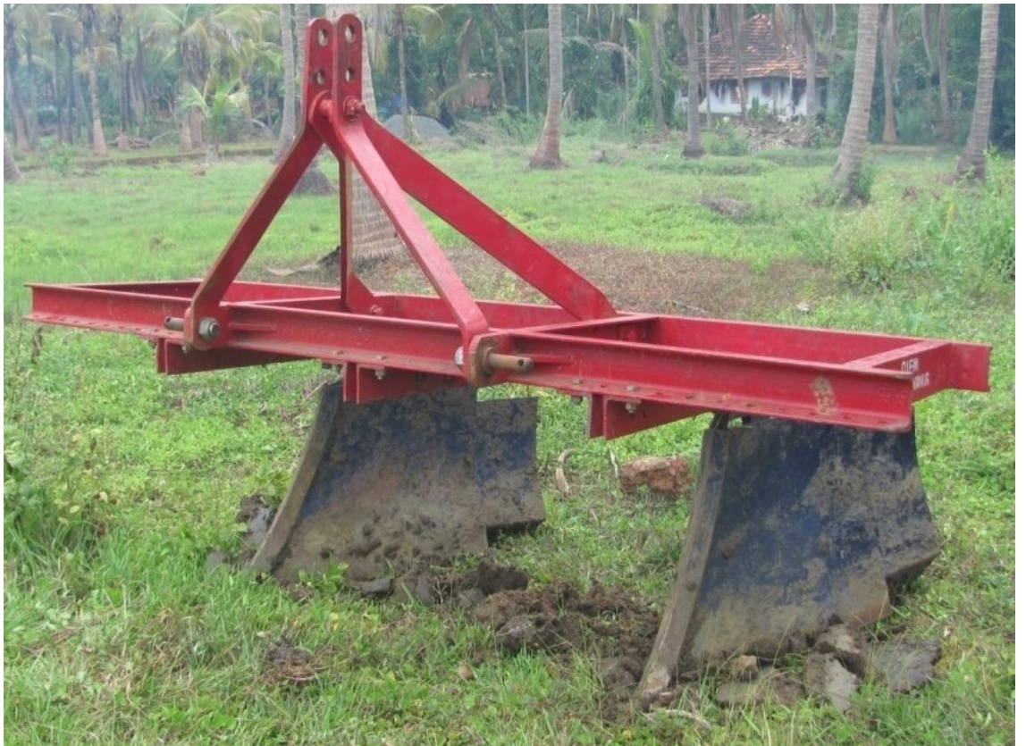
Plate. 3. 2. Tractor operated Kaipad bed former
