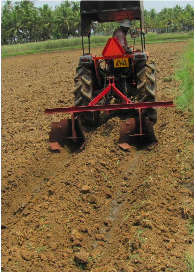
Plate. 3. 5. Field performance of tractor operated Kaipadbed former
