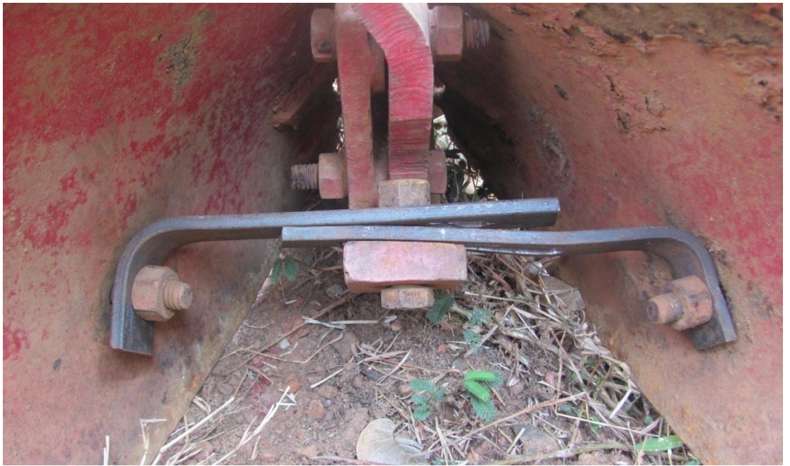
Plate. 3. 3. Angle adjustment of the plough bottom
