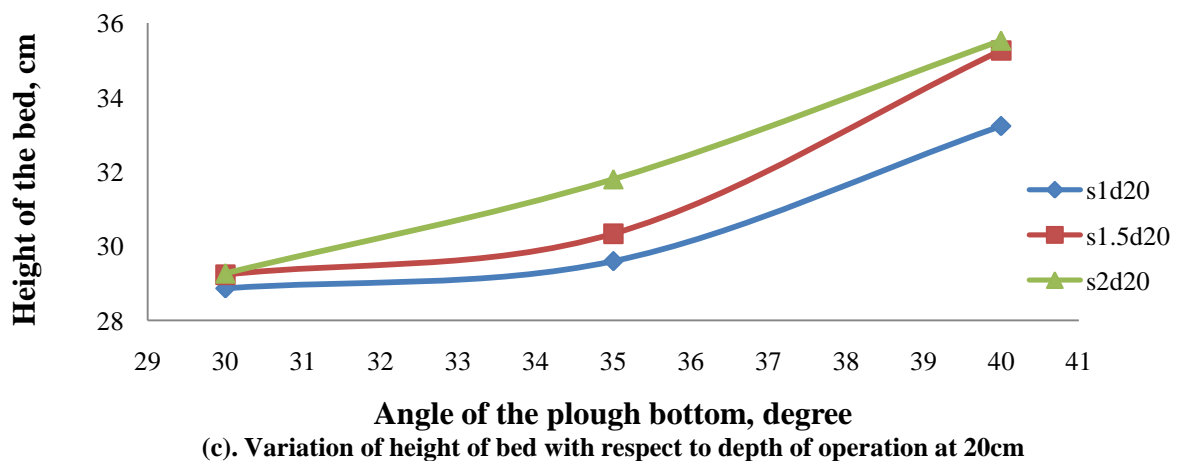
Fig. 4.2. Effect of height of bed at different angles of plough bottom, different speed and depth of operation
