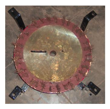
Plate 3.3 Polyurethane (Grinding surface)
