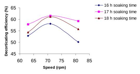
Fig. 4.13 Decorticating efficiency Vs Speed for grinding stone at different soaking time
