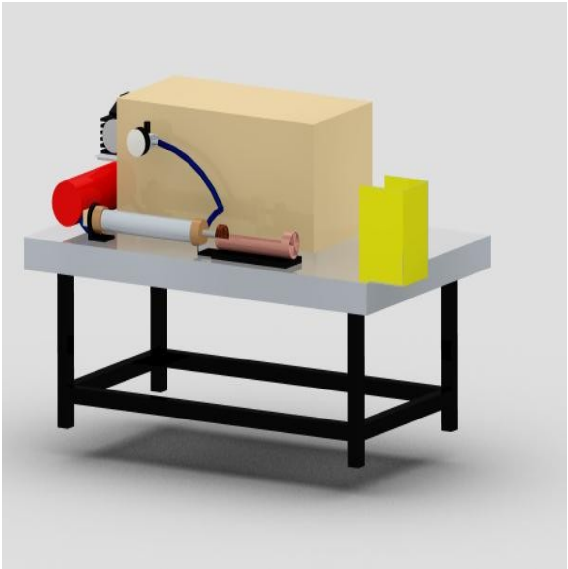
Plate 3.14. Schematic isometric view of pneumatic potato slicer
