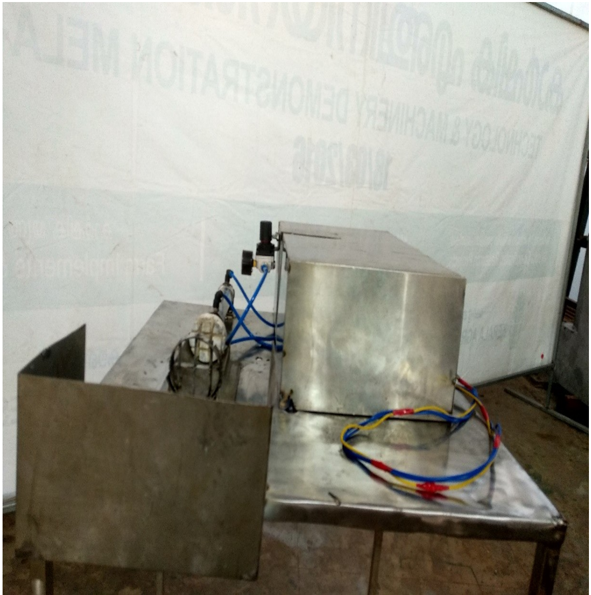
Plate 3.12. Side view of pneumatic potato slicer
