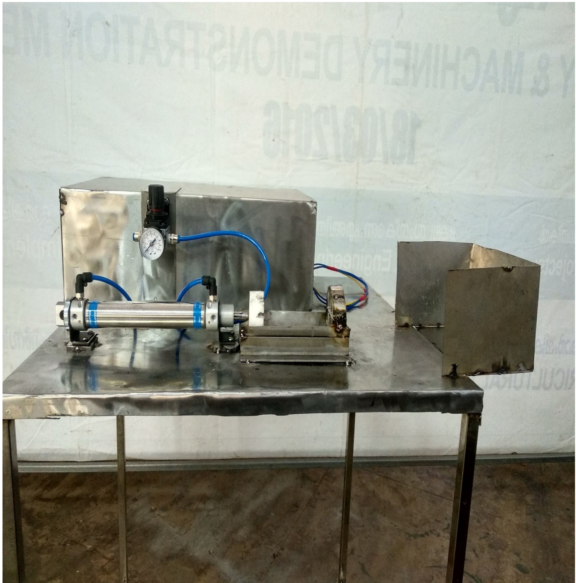
Plate 3.11. Front view of pneumatic potato slicer
