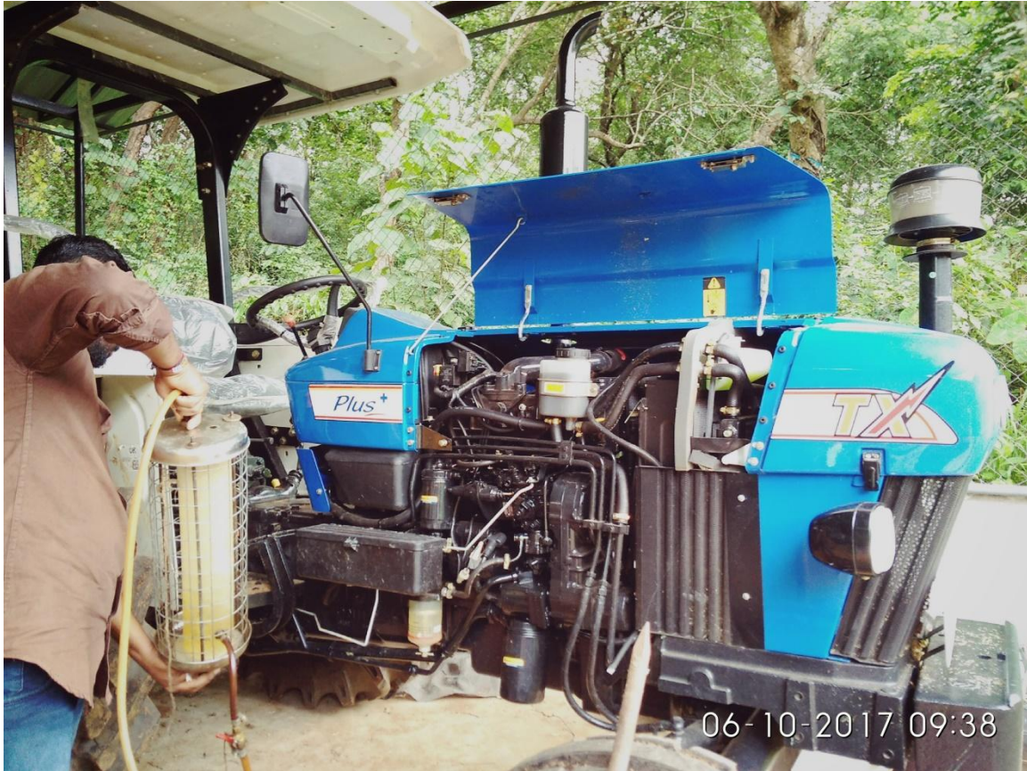
Plate 3.6 Installing fuel jar for measuring fuel consumption
