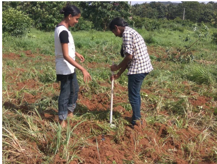
Plate 3.2 Core cutter method
