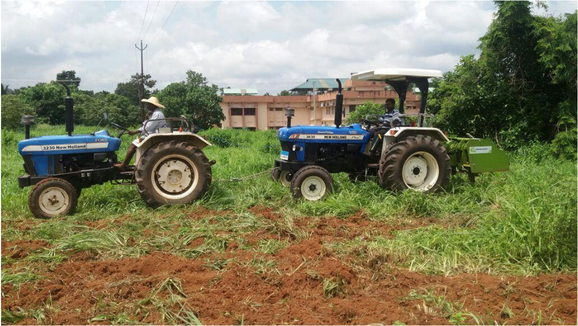
Plate 3.8 Two tractor method for draft measurement
