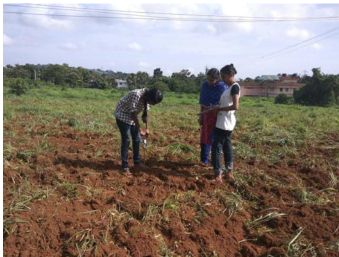
Plate 3.5 Measurement of penetration resistance using cone penetrometer
