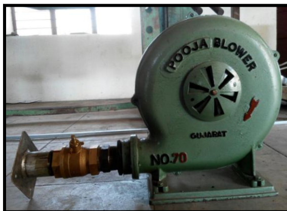
Plate 3.2. Blower with flow control valve
