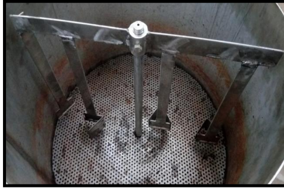
Plate 3.3. Agitator inside drying chamber
