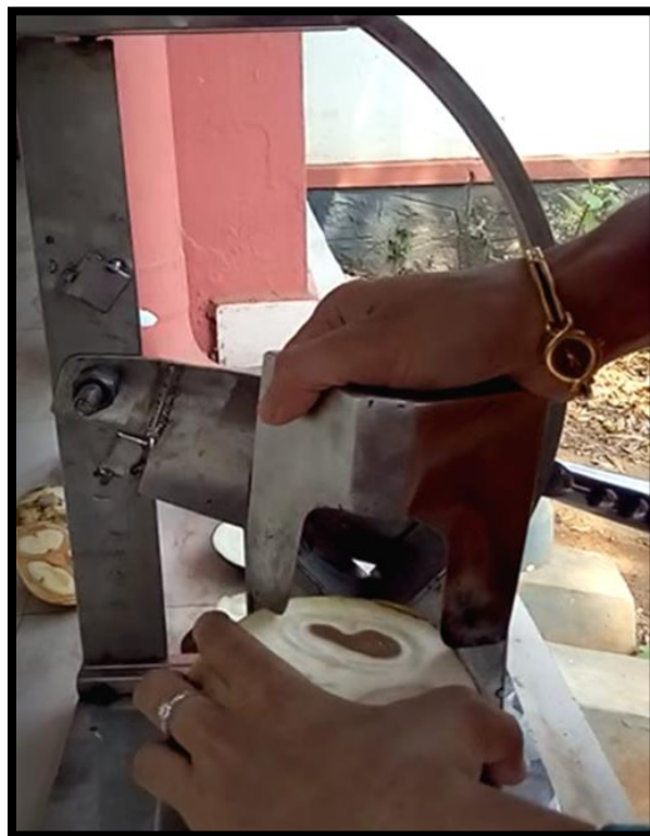
Plate 4.5. inserting Blade into Fruit
