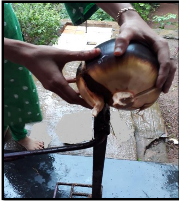
Plate 3.1 palm fruit open using Keramithra tool
