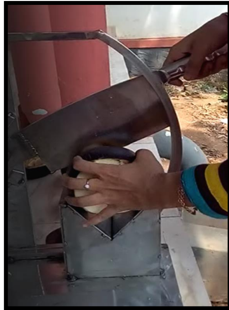
Plate 4.4. Cutting top side
