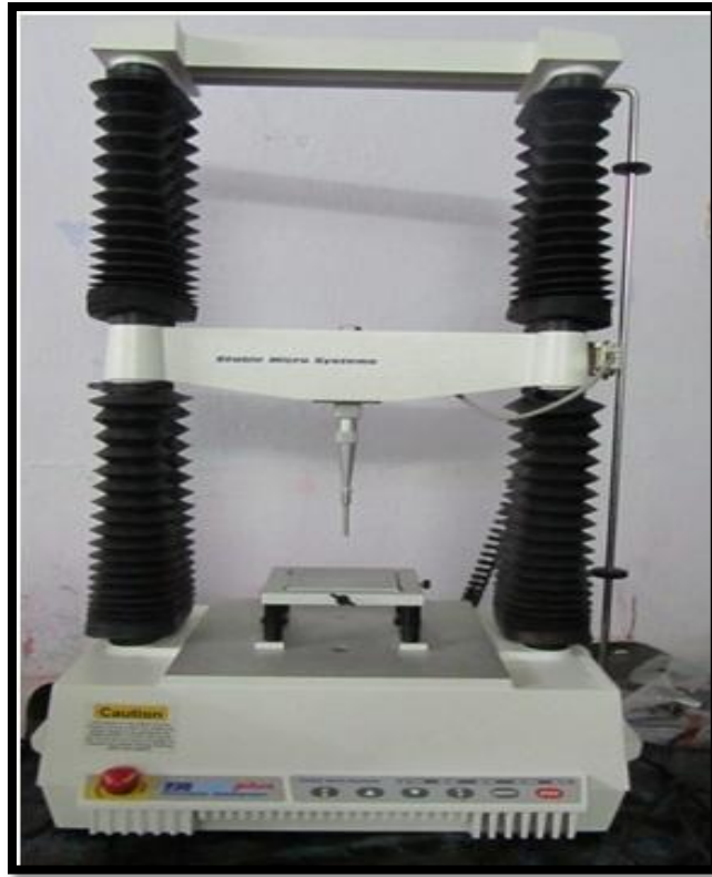
Fig.3.2 Texture analyser (Stable Micro Systems)
