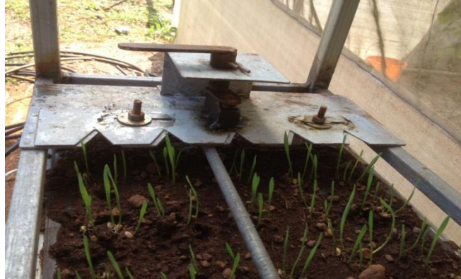
Plate 3.5 Fabricated fodder cutting mechanism suitable for tray cultivation
